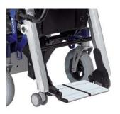
The foot plates can be swivelled up for easy transfer.
