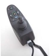
The joystick is programmable for individual needs and preferences. It is also easy to read and operate.
