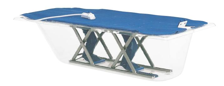
With its large lying area, the full-length platform bath lift Aquatec Major offers the optimal solution for users who can only bath in lying position. It is custom-made to the dimensions of the bathtub and thus ensures the maximum safety during transfer. The platform bath lift is operated hydraulically and can be obtained for three weight classes: 20 - 70 kg, 50 - 130 kg, 100 - 150 kg. The removable and machinewashable cover is available in white or blue.
