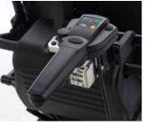
Allows access to the drive function, speed dial, forward and reverse option and speed handle with emergency stop feature. It also indicates who is in control, the on/ off status and the forward and reverse status.
