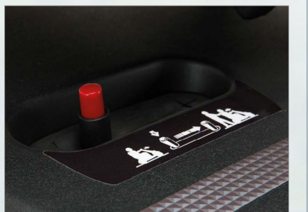
Two-step disengaging lever to prevent free-wheeling
