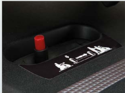
Two-step disengaging lever to prevent free-wheeling
