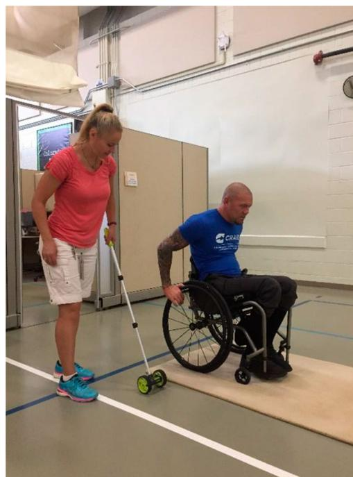
**Figure 6 One Stroke Push – The forward distance propelled when pushing once with maximal effort on carpet was measured. This evaluates single stroke propulsion efficiency and is a functional mobility measure.**
