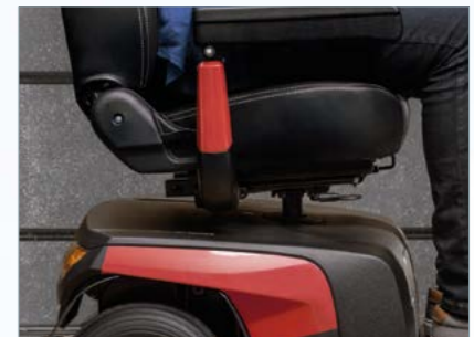
Reinforced seat column
