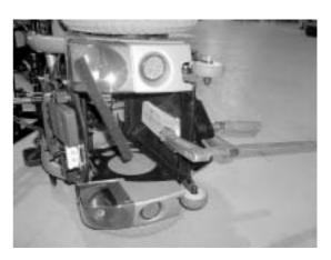
The docking station fixing has four drill holes for fixing, two at the rear (1) and two at the front (2). You can use these holes as a drill template.
