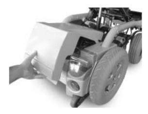
• Remove plastic clips (1) and remove the equipment rack upwards to the rear.
