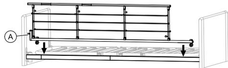
Place the side rail over the top frame with the release system (A) at the head end of the bed.
