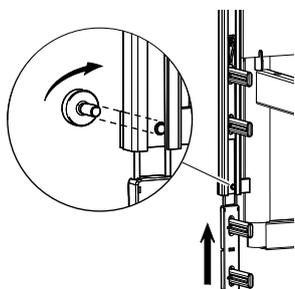
Loosen the screw at the bottom of the guides on one of the bed ends and push the glider halfway up into the guide until it attaches with an audible click.
