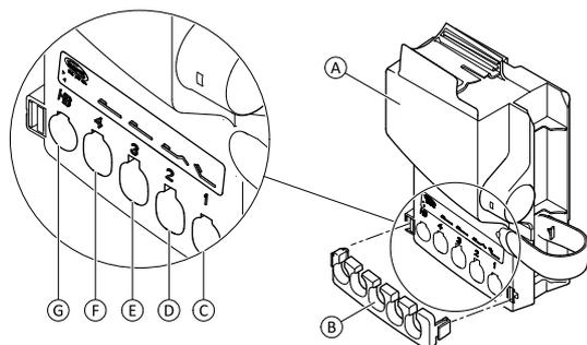
The control box (A) is provided with a locking cam (B) and a label with symbols showing where to connect the motor plugs:
