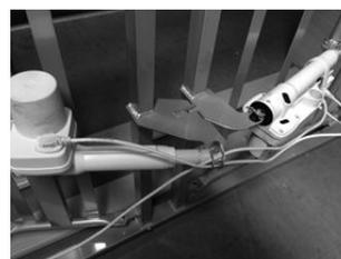
Guide the hi/lo motor cable from the bed foot end and the cable from the thigh/leg section motor through the thigh/leg section motor pipe pin. Make sure the pipe pin is properly locked.
