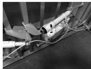
Connect both plugs from the hi/lo motors (head end and foot end) to the control box placed underneath the backrest.
