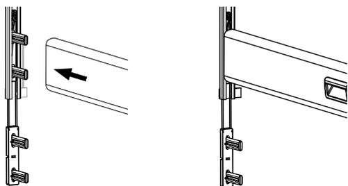
Push the upper side rail onto the two upper pawls.
