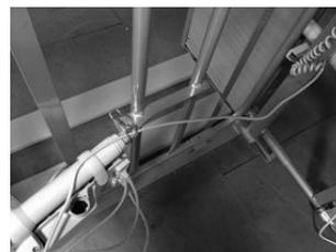
Place the cable from the hi/lo motor in the head end, on the two hooks at the bed end and attach the cable in the backrest motor pipe pin.
