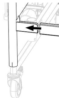
Push the bed side tubes onto the bed end attachment. Make sure it is all the way in.
