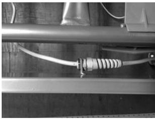
Attach the mains cable in the strain relief that is attached to the bed frame.
