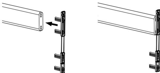
In the other end of the side rail bar; push the two upper pawls into the end of the bar.
