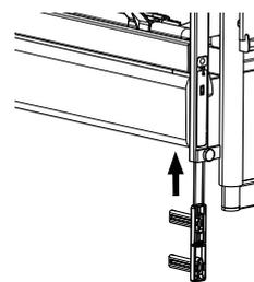
Push the attachment into the guide until it attaches with an audible click (=properly engaged in the lower position).
