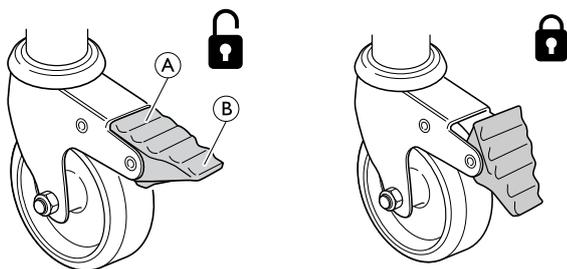
**Locking the brake** - Step on the outer part **B** of the brake pedal
