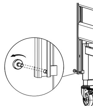
Retighten the screw under the lower side rail bar, in each corner of the bed ends.
