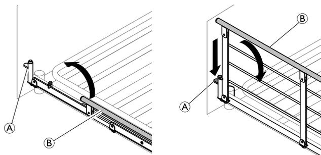
1. **Up:** Lift and pull the top bar **B** of the side rail towards the end with the locking mechanism (release button) **A**. Ensure, it is locked in place.
