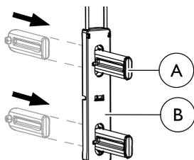
Push the pawl **A** from the backside, through the glider **B** and make sure it locks with an audible click.
