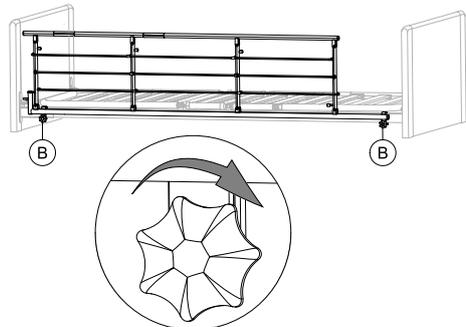
Tighten the finger screws (B) to attach the side rail on the top frame. Make sure it is steady and fastened.
