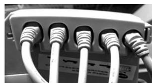
Install the locking cam over the plugs in the control box.
