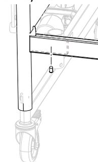
Fasten the bed end side tubes with the screws and make sure they are properly tightened.
