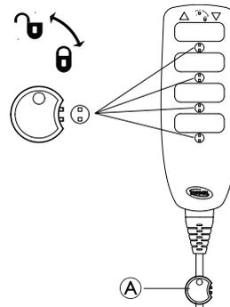
1. Insert key (A) in the key hole, below the wanted function.
