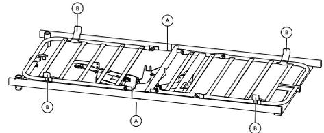
Tighten with the two thumb screws (A) (one on each side).
