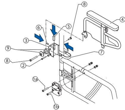
**i** The sleeves ⑨ are different for flip to back side rest in frame colour and flip to back side rest with engagement mechanism.
