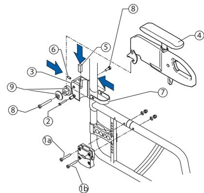
**i** The sleeves ⑨ are different for flip to back side rest in frame colour and flip to back side rest with engagement mechanism.
