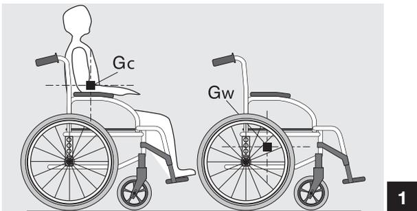
You will remain stable in the wheelchair whilst the line of your combined centre of gravity lies within the points of contact of the forward and rear wheels with the ground.
