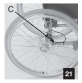
To adjust braking : turn the screw (C) counterclockwise to increase braking force and turn clockwise to reduce it.
