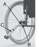
Make sure that the dog points locates in and protrudes through its appropriate location hole in the frame tube in order to prevent any falls.
