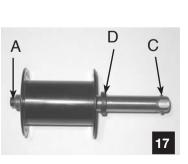
Always make sure that the spacer (D) is in place. Make sure that the axle and the locking balls are clean. (wipe out every month with a rag soaked with fine oil)
