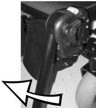
Swivel the legrest upward in order to access the rubber stop.
