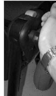
Hit the knob to release the locking mechanism.
