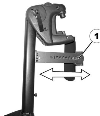
1. Use the wrench to loosen the nut (1) and remove.
