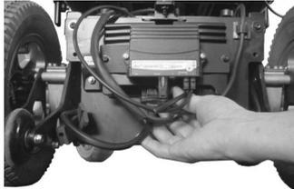
Disconnect the battery cable from the electronic module.
