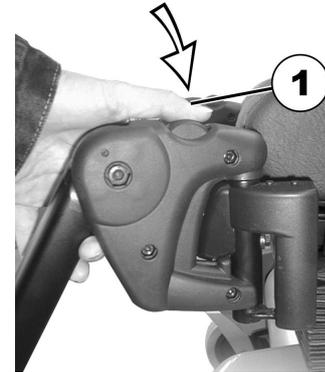
1. Press the unlocking button (1) and swivel the footrest/legrest outward.
