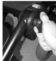
Turn the knob clockwise to tighten it.
