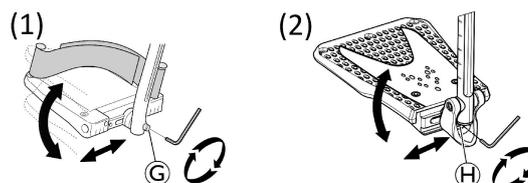
1. Loosen the fixing screw G or H with 5 mm Allen key.
