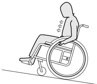
1. Bend your upper body forwards and propel the wheelchair with quick, powerful strokes on both handrims.
