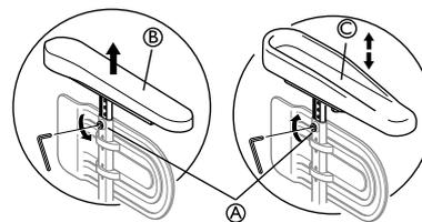
1. Loosen the screw (A).
