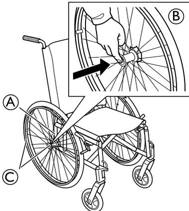
1. Press and hold in the quick-release button **B** in the center of the hub.
