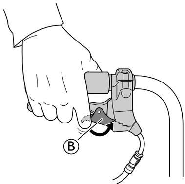
Pull the brake handle upwards and push the lock catch **B** downwards to lock the brake.
