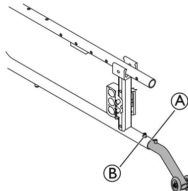
1. Remove the plastic plugs from the end tube of the chassis (A).
