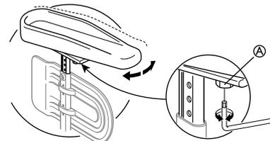
5. The hemiplegic armrest can be adjusted in angle. The resistance can be increased/decreased by adjusting the screw (A).
