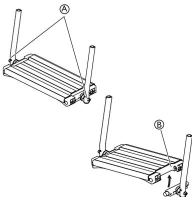
1. Adjust the angle and the depth by loosening the two screws © at the foot plate attachment.
