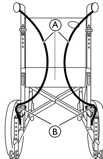
1. Fold the cables **A** inwards as shown on the picture.
