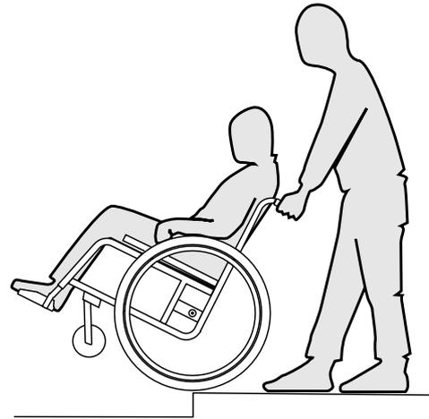
1. Move the wheelchair right up to the kerb and hold the handrims.
