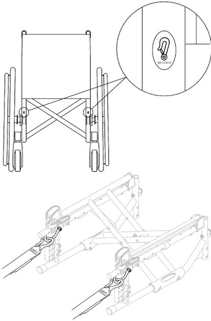
1. Attach the snap hooks to the orange rings as shown in the two figures above (see location of the attachment labels).
