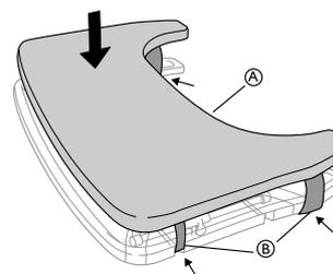
Place the cushion for the table tray (A) on the table and place the attachment straps (B) around the table.
