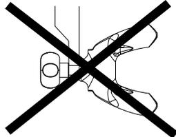
Make sure that the hand wheel for the push handle (A) fits the hole in the tubes. If the threaded tap of the hand wheel (B) is more than app. 2.5 mm visible, the position is wrong. Lower or raise the push handle to get the hand wheel in the correct position.
