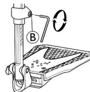
1. Loose the fixing screw B with 5 mm Allen key.
