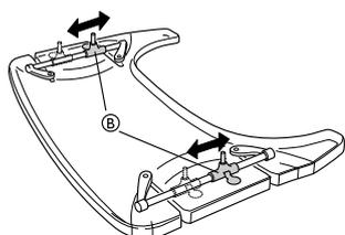
Adjust the table holders (B) forwards or backwards to adjust to the required depth.
