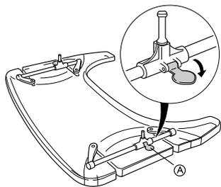
Open the safety lock for the depth adjustment (A).
