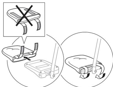
1. Thread the foot plate cover onto the foot plate.
