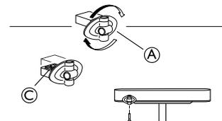
To fit the table attachment (A) to the wide armrest, turn the attachment around, the patterned surface (C) should now be facing upwards.
