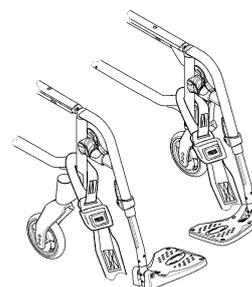
1. Attach the front straps above the castor supporters as shown in the figure above (see location of the attachment labels).
