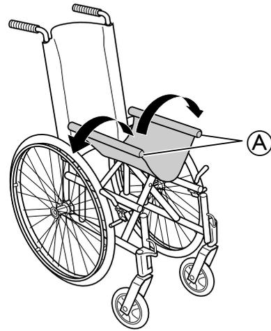
Press the seat edges **A** outwards / downwards to unfold the wheelchair.
