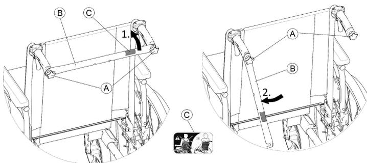
1. Slightly loosen the two hand screws A, pull up the backbrace B and swivel it downwards along the backrest (on right or left hand).
