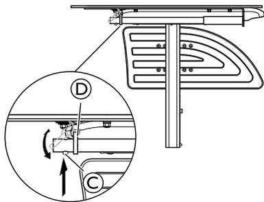
2. Push on the push pin (C) and insert the ring (D) on the tube (A).
