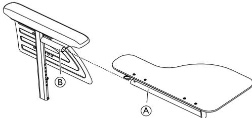
1. Insert the tube of the half tray (A) into the attachment (B) under the arm pad.
