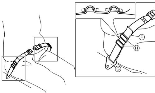
1. Thread the loop **F** through the fixation on the chair **G** and then through BOTH plastic buckles **H**.
