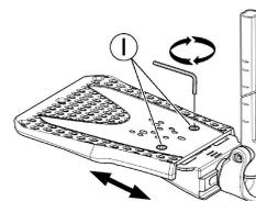
1. Loosen the two fixing screws I with 5 mm Allen key.
