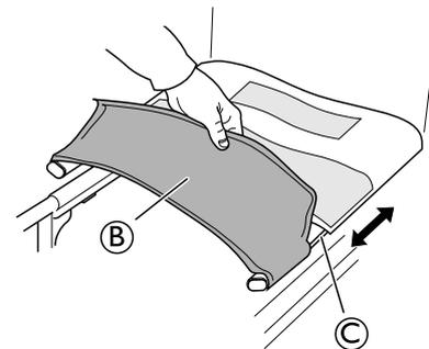
Release the front part of the seat (B) from the hook and loop strips.
