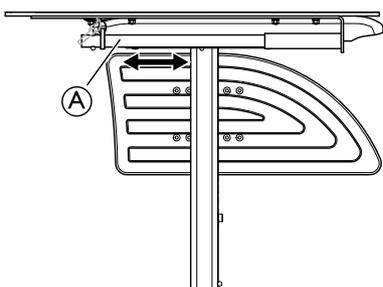
1. Slide the half tray (A) forwards or backwards to adjust to the required depth.
