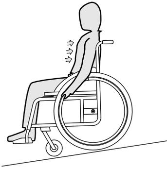
1. Lean back and carefully allow the handrims to run through your hands. You should be able to stop the wheelchair at any time by gripping the handrims.
