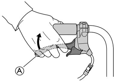
Pull both brake handles upwards to engage the brake.
