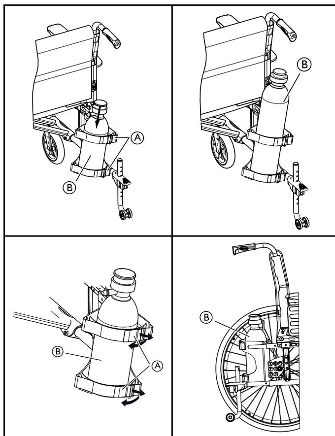
1. Loosen the hook and loop strips **A** on the rear of the O<sup>2</sup> holder by simply pulling on them.
