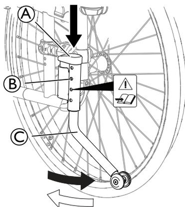
1. To adjust the height, press on the two knobs (B) placed on each side of the housing.
