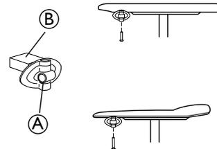
Mount the table attachment (A) with the attachment part facing outwards. The plain surface (B) of the attachment should be placed upwards when using the table on the thin armrests.
