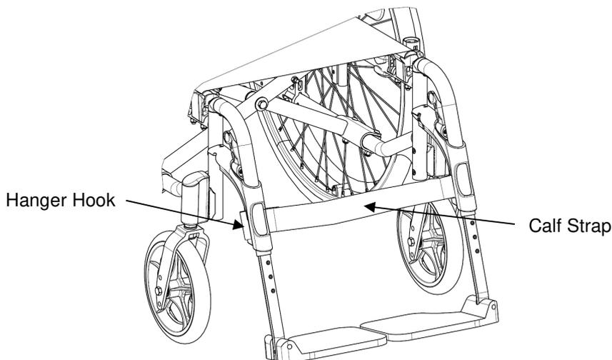
**FIGURE 2.3** Installing Calf Strap
