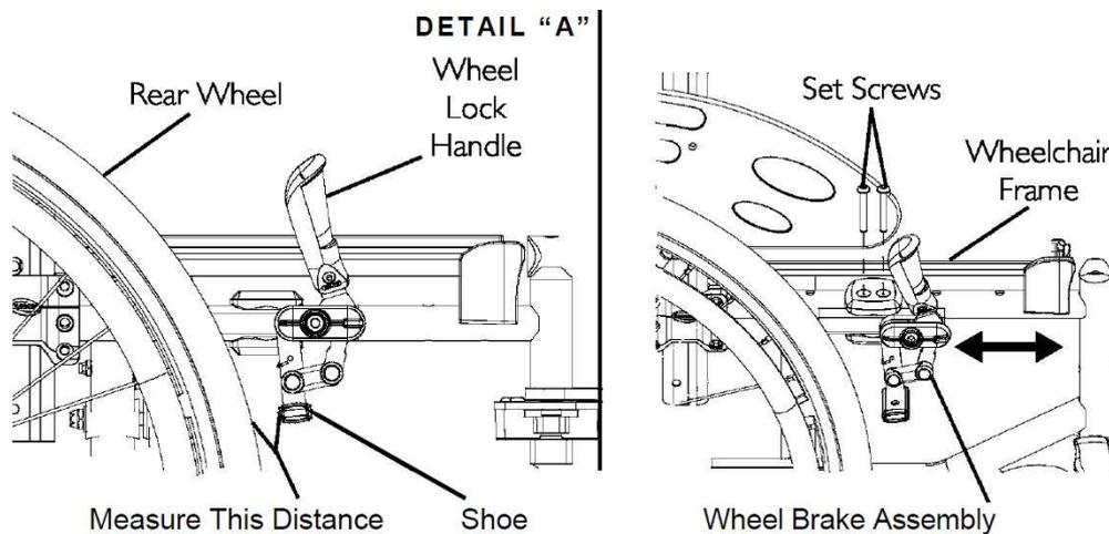
**FIGURE 7.2** Adjusting Wheel Brakes- Adjusting Wheel Brake Tension
