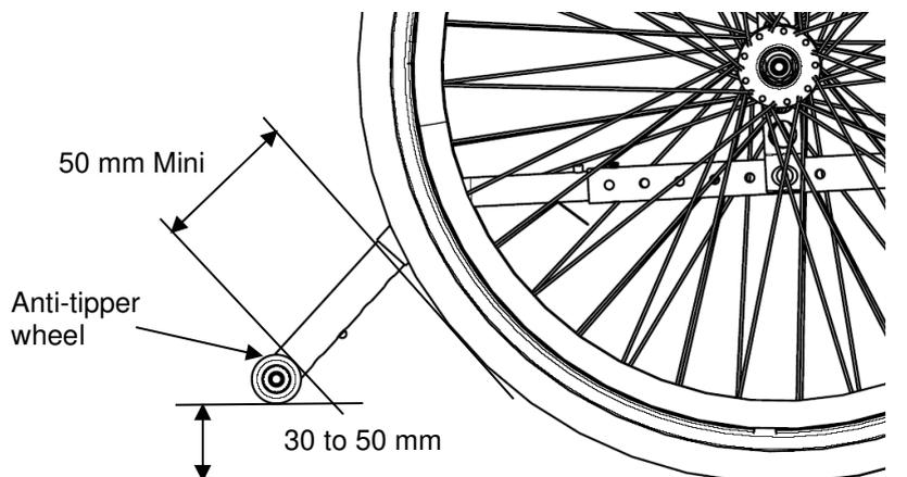
**FIGURE 9.3** Adjusting Anti-Tippers
