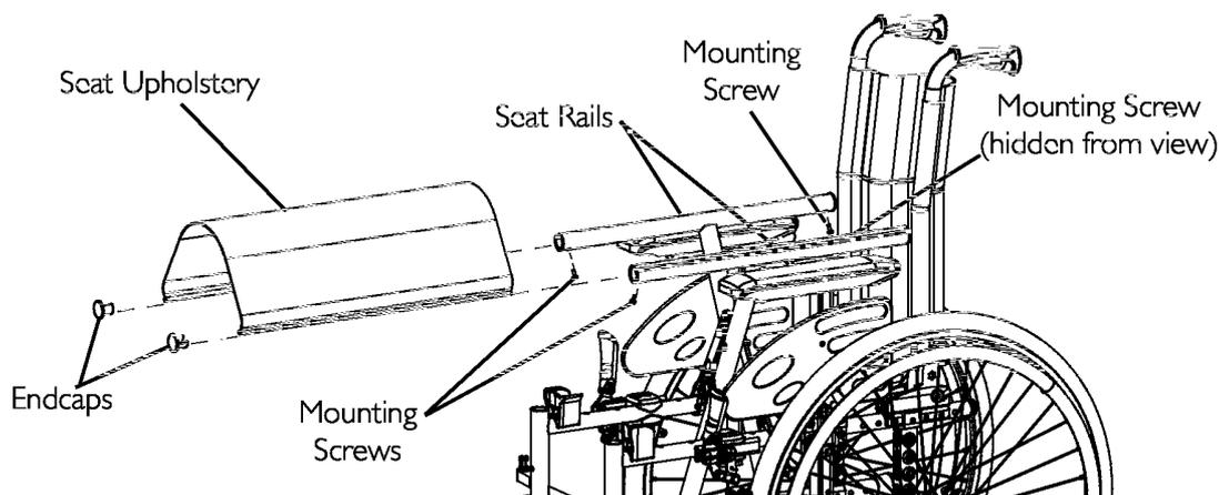
**FIGURE 4.2** Removing/Installing Seat Upholstery
