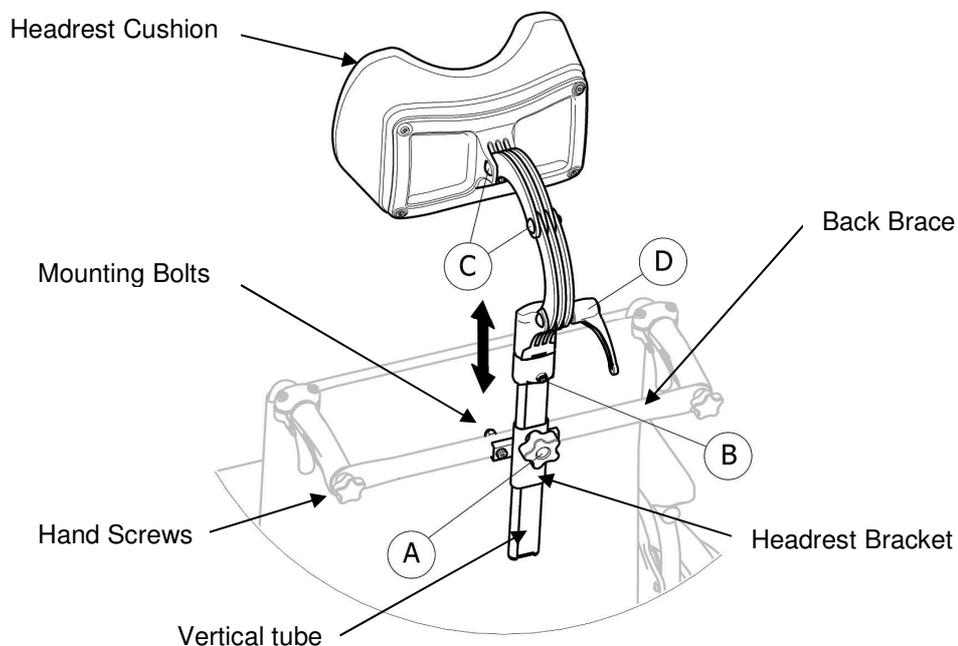
**FIGURE 8.2** Installing Headrest
