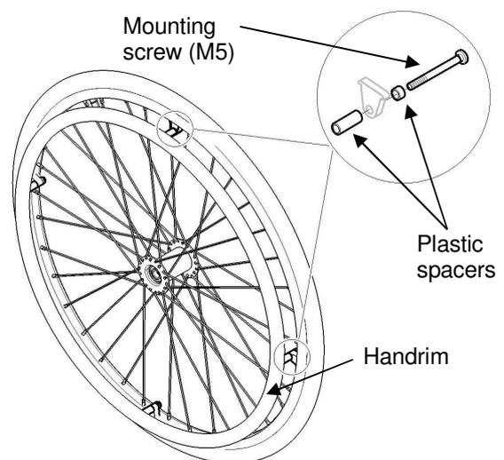
**FIGURE 5.4** Replacing Handrims
