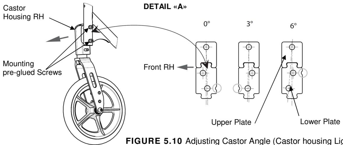
**FIGURE 5.10** Adjusting Castor Angle (Castor housing Light)
