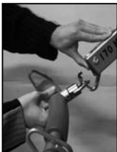
Easy opening of the carabineer by pushing the safety catch backwards with one finger and attachment of the spreader bar.
