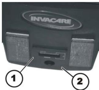
The operating hour counter is located on rear shroud (2).
