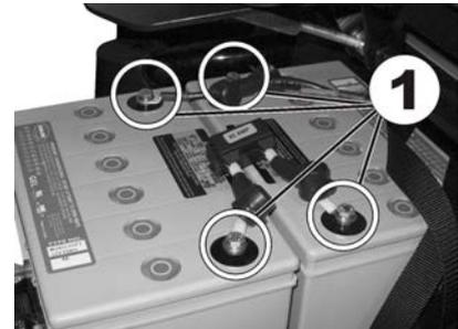
Remove the terminal cover from the battery terminals (1).
