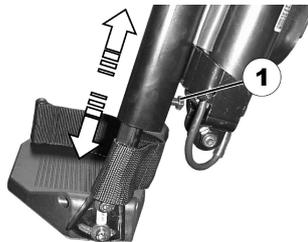
1. Use the wrench to loosen the screw (1).
