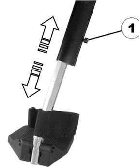
1. Use the spanner to loosen the screw (1).
