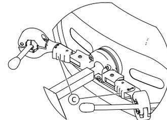
Press locking device **C** (behind headrest) and swivel joystick or egg switch inwards or outwards until it clicks in place.
