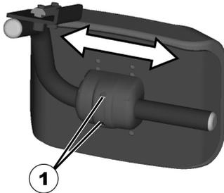
1. Loosen the Allen screws (1) using the Allen key.
