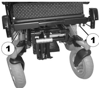
The screws that allow width adjustment of side-mounted legrests are located under the seat (1).
