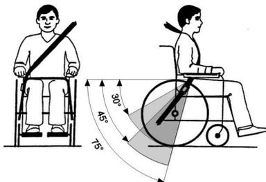
The pelvic belt should be positioned in the area between the user's pelvis and thighs so that it is unobstructed and not too loose. The ideal angle of the pelvic belt to the horizontal is between 45° and 75°. The maximum permissible angle is between 30° and 75°. The angle should never be less than 30°!
