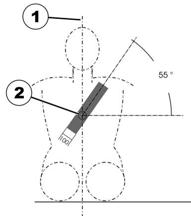
The safety belt installed in the transporting vehicle should be applied as shown in the illustration above.
