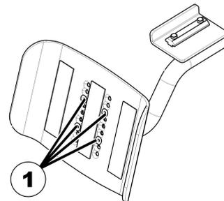
Loosen the screws (1) using the crosstip screwdriver and remove them.
