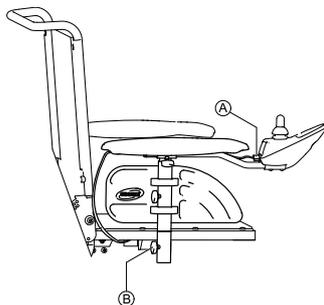
1. Pull the plug **A** of the remote cable to disconnect the remote.
