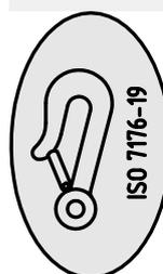
3. The tie-down points on the wheelchair where the restraint system straps should be placed are marked with this symbol.
