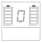
Push the button [24] on the remote control to simultaneously switch off both e-motion wheels. A zero and the charge status of both battery packs is indicated in the display. A beep sounds at the e-motion wheels.
