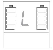
When activating the button lock, the following is shown in the display: the current charge status of the two battery packs, an "L" in alternating fashion, the power stage currently set (1 or 2) and in case an error occurs, the corresponding error code.
