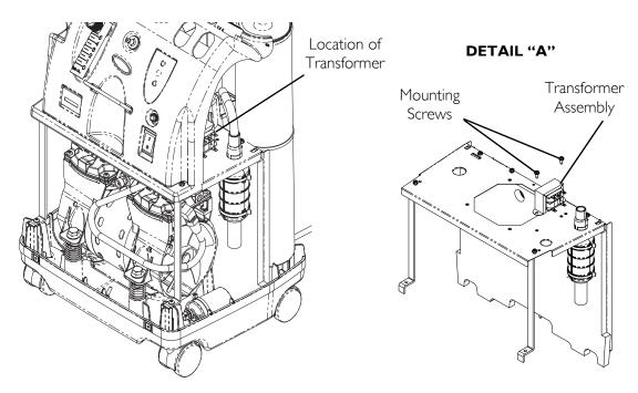
FIGURE 16.1 Replacing the Transformer
