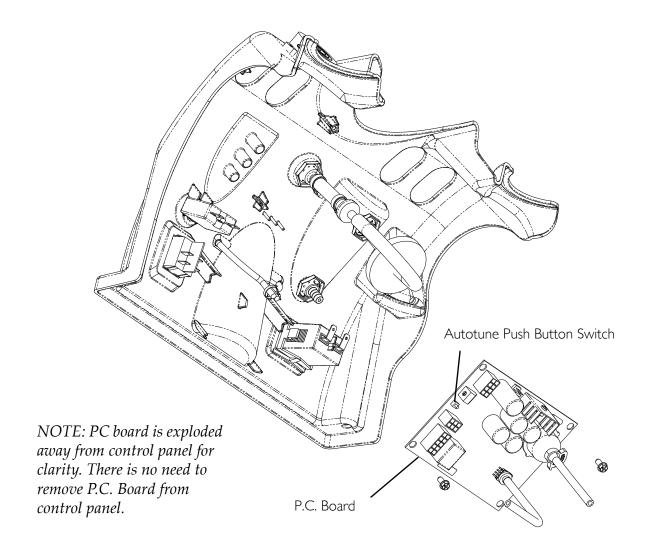
FIGURE 22.1 Autotuning (Model IRC5PO2AW Only)
