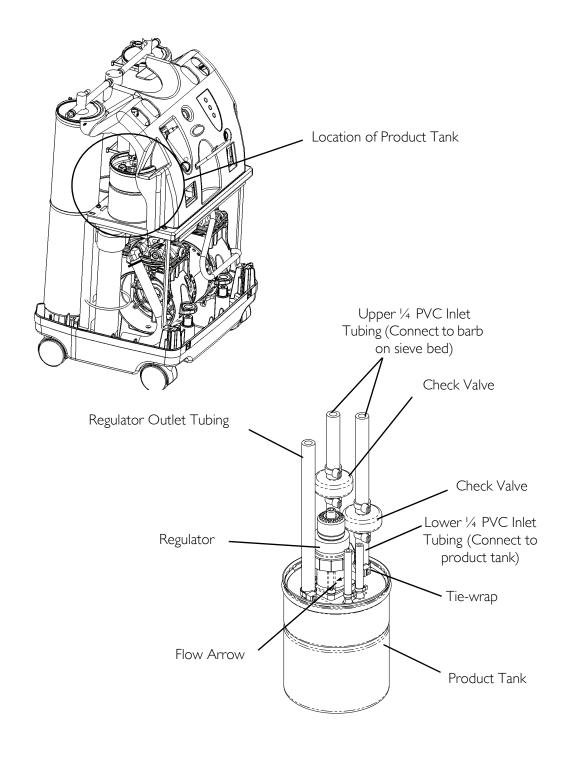
FIGURE 10.1 Replacing Check Valves
