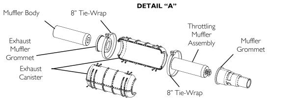
FIGURE 6.5 Replacing the Muffler Assembly
