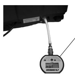
Use a 0-206.84 kPa (0-30 p.s.i.) pressure gauge to monitor system pressure swings, and also record the amount of time it takes / to achieve a shift (full charge and full purge).
