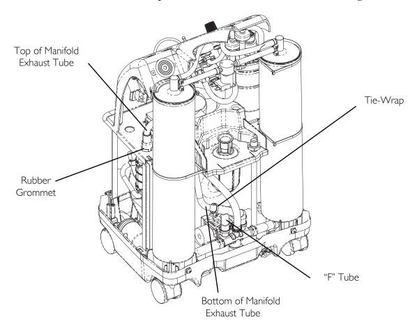
FIGURE 6.4 Replacing the Muffler Assembly
