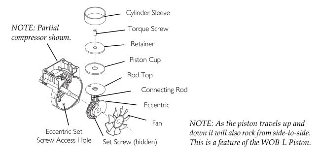
FIGURE 7.4 Removing Compressor and Compressor Heads - Rebuilding the Compressor - Fan - Connecting Rod and Eccentric Assembly - Piston Cup
