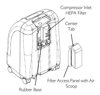
FIGURE 6.3 Replacing the Compressor Inlet HEPA Filter
