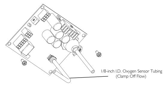
FIGURE 24.3 Oxygen Sensor
