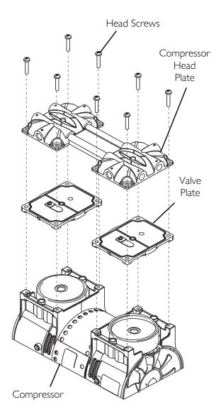
FIGURE 7.3 Removing Compressor and Compressor Heads - Rebuilding the Compressor - Compressor - Compressor Head Plate - Valve Plates
