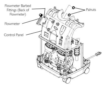
FIGURE 18.1 Replacing Flowmeter
