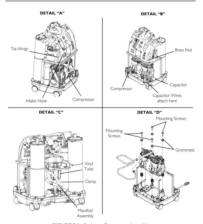
FIGURE 7.1 Replacing Compressor Assembly
