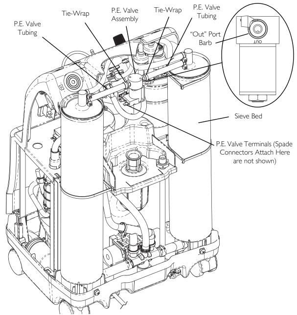
FIGURE 8.1 Replacing P.E. Valve
