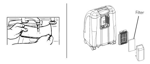
FIGURE 6.1 Cleaning the Cabinet Filter
