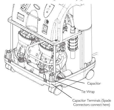
FIGURE 7.2 Replacing Capacitor
