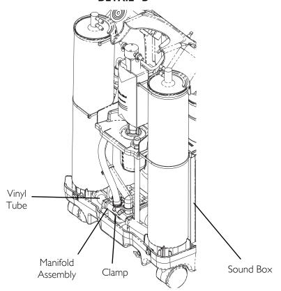
FIGURE 12.1 Replacing Heat Exchanger Assembly
