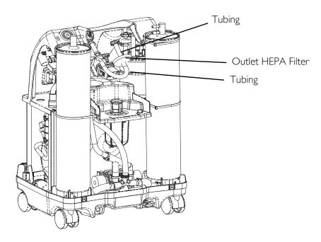
FIGURE 6.2 Replace the Outlet HEPA Filter
