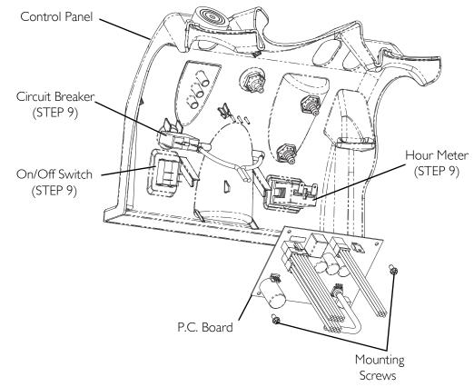
FIGURE 13.1 Removing Control Panel
