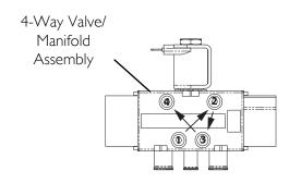
NOTE: The numbers above indicate the mounting screw torque sequence: pre-torque to 1.1 N-M  $\pm$  0.2 N-M (10  $\pm$  2 inch-lbs), then torque to 2.5 N-M  $\pm$  0.2 N-M (22  $\pm$  2 inch-lbs).
