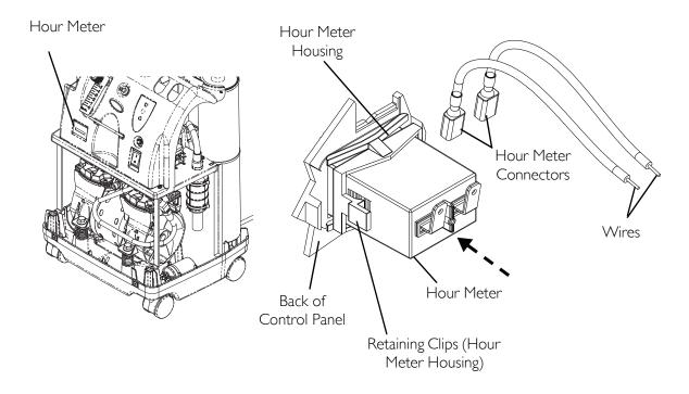
FIGURE 19.1 Replacing Hour Meter
