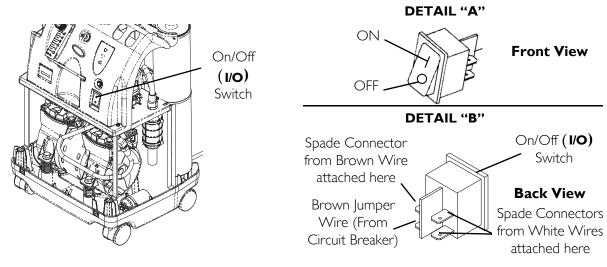
FIGURE 17.1 Replacing On/Off Switch
