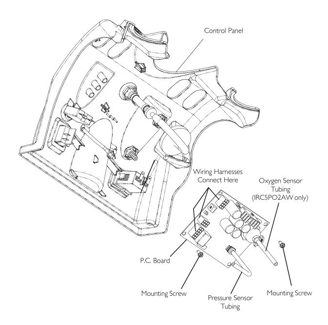
FIGURE 15.1 Replacing P.C. Board
