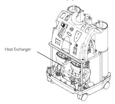
FIGURE 6.6 Cleaning the Heat Exchanger
