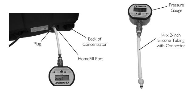
FIGURE 25.2 Pressure Testing
