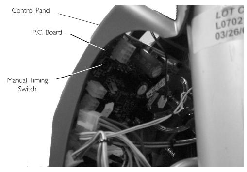
FIGURE 22.2 Manual Tuning (Model IRC5PAW Only)
