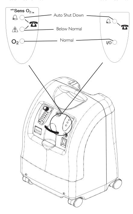
FIGURE 21.1 Display Control Panel
