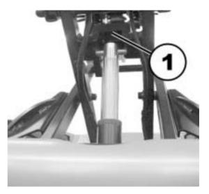
• Raise the seat slightly and release the holding mechanism (1). Lower the seat slowly until the weight of the lifter is resting on the actuator again.
