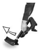
• Lowering: Keep the legrest in the foot plate area, pull the lateral adjusting lever (1) and lower the legrest slowly.
