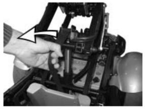
• One person now pulls the seat upwards, and a second person ensures that the actuator bolt head (1) is guided out of its mounting and does not jam.
