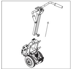
Remove the hand grips from the drive unit, as shown in the figure.
