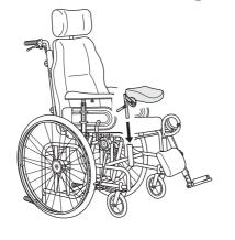
**I.** Remove the existing footrest and fit the amputee legrest in its attachment.
