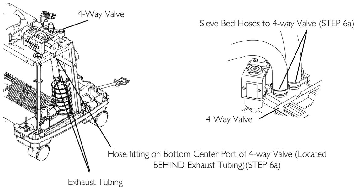
**For 5 Liter Models with Throttle Muffler (manufactured after 7/24/03)
