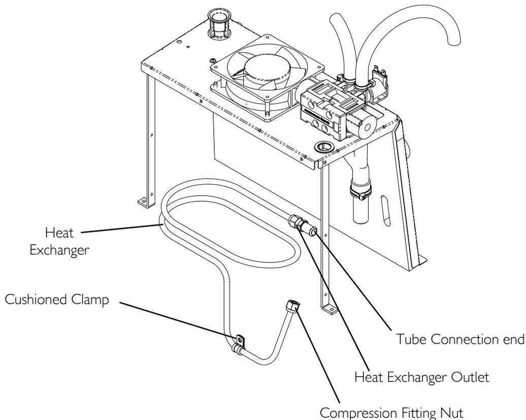
**FIGURE 12.2** Replacing Heat Exchanger - Platinum 5 Models Manufactured After 9/9/2005
