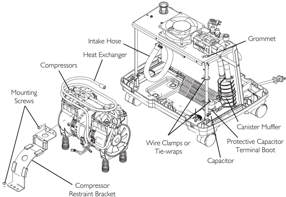
**FIGURE 7.1** Replacing Compressor Assembly - 5 Liter Models manufactured before July 24, 2003
