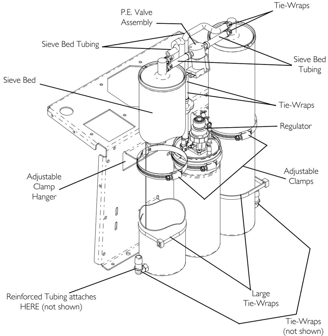
**FIGURE 9.1** Replacing Sieve Beds - 5 Liter models manufactured before 1/27/05
