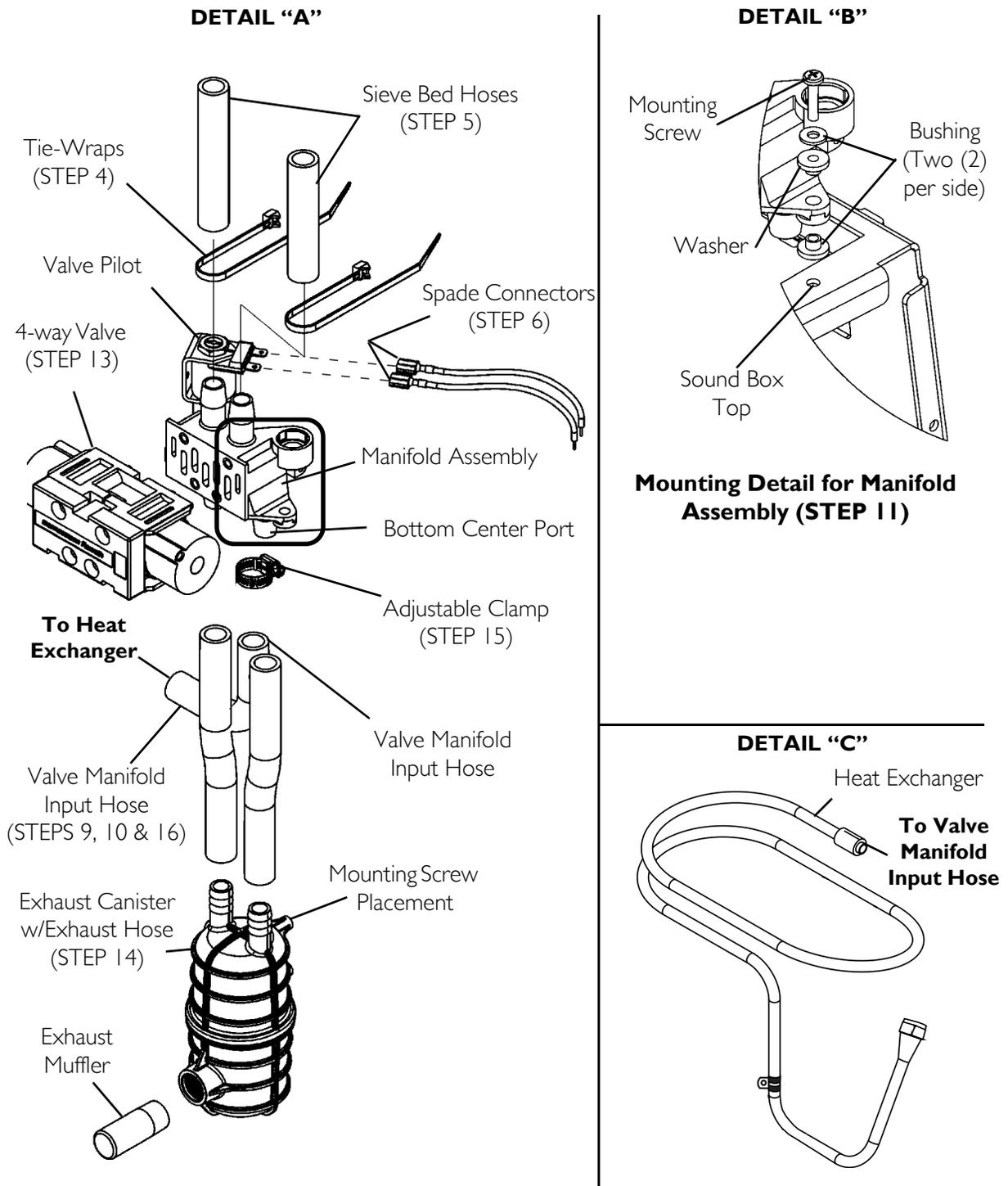
**FIGURE 20.3** Replacing Manifold Assembly- 5 Liter Models Manufactured before 7/24/03
