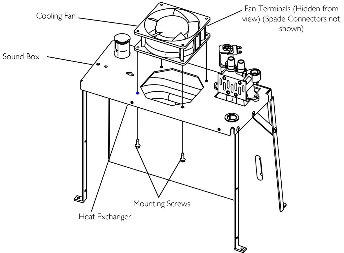
**FIGURE 14.1** Replacing Cooling Fan
