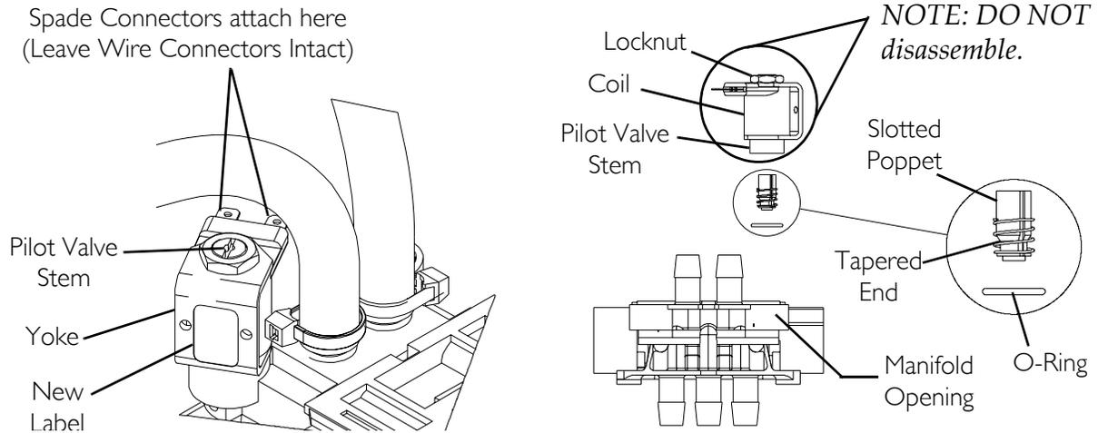
**FIGURE 20.5** Replacing Pilot Valve Poppets and O-Rings - 5 Liter Manufactured Before 8/1/05
