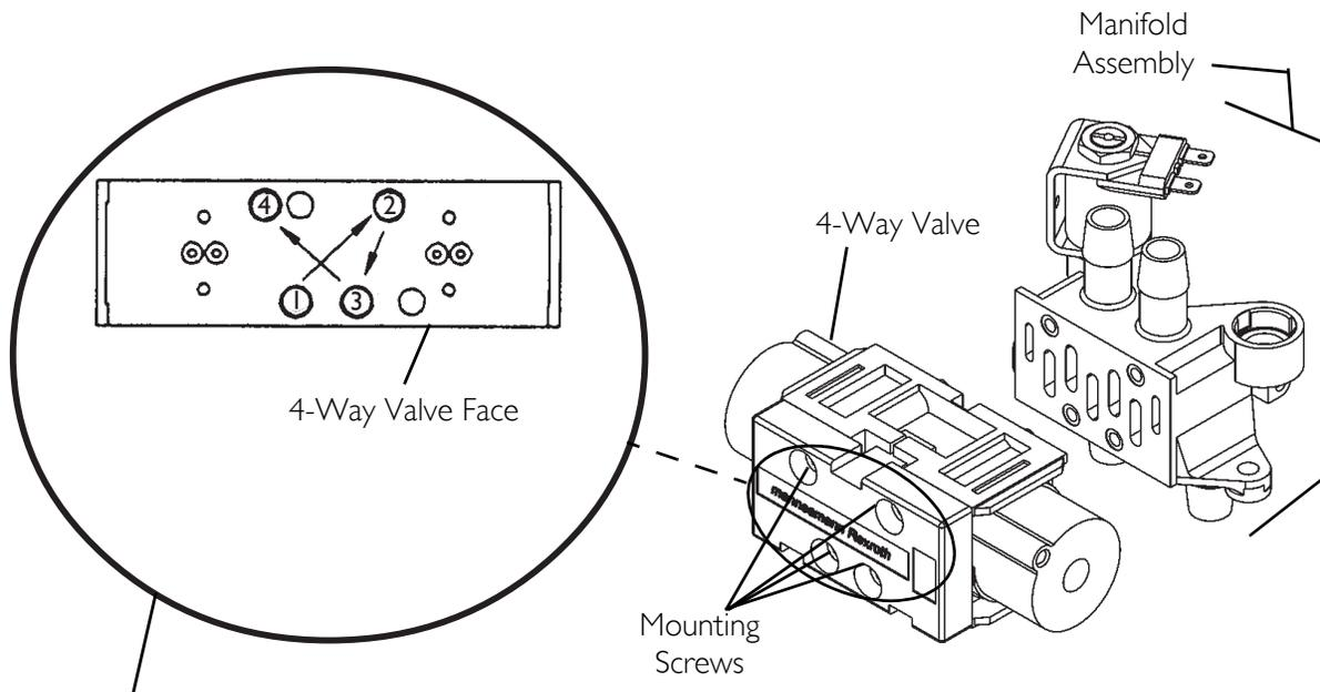
*NOTE: The Numbers indicate the mounting screw torque sequence: pre-torque to 1.1 N-M  $\pm$  0.2 N-M (10 in-lbs  $\pm$  2 in-lbs), then torque to 2.5 N-M  $\pm$  0.2 N-M (22 in-lbs  $\pm$  2 in-lbs).*
