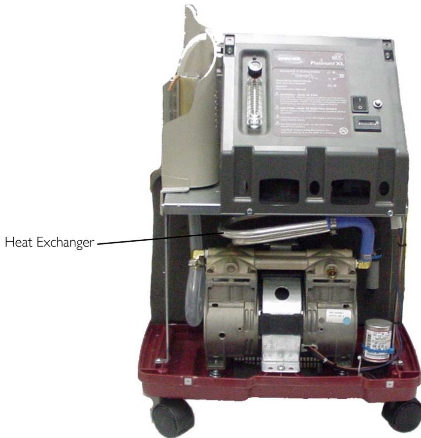
**FIGURE 6.8** Cleaning the Heat Exchanger
