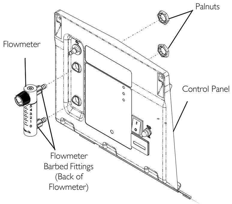
**FIGURE 18.1** Replacing Flowmeter
