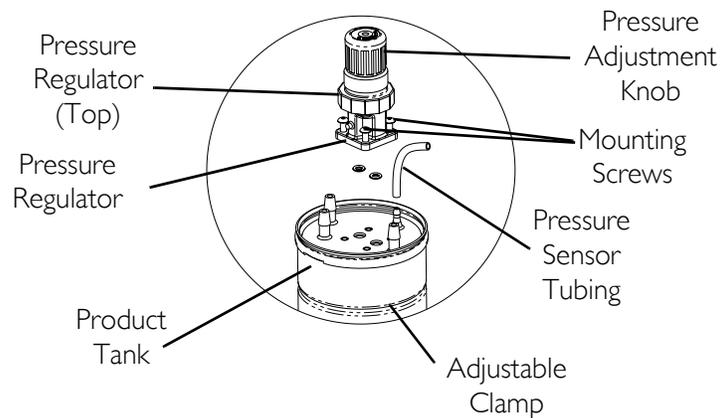
**FIGURE 11.1** Replacing/Adjusting Regulator
