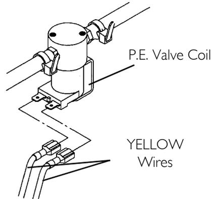
**FIGURE 24.4** P.E. Valve Coil Test
