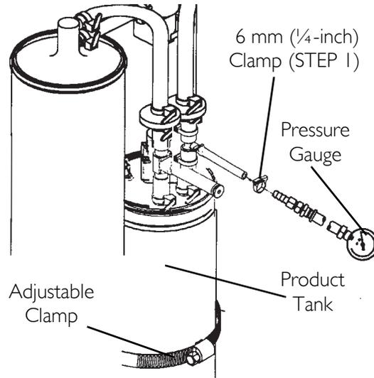
**FIGURE 25.3** Pressure Testing
