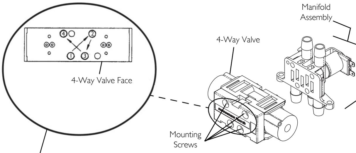
*NOTE: The Numbers indicate the mounting screw torque sequence: pre-torque to 1.1 N-M  $\pm$  0.2 N-M (10 in-lbs  $\pm$  2 in-lbs), then torque to 2.5 N-M  $\pm$  0.2 N-M (22 in-lbs  $\pm$  2 in-lbs).*
