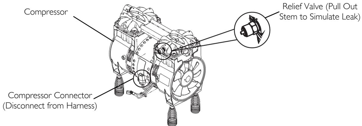
**FIGURE 24.1** Low Pressure Test - Time-Out Test
