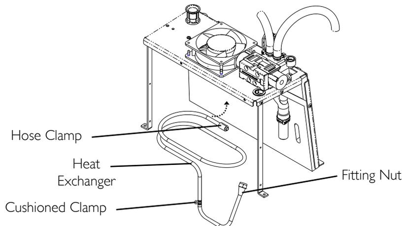
**FIGURE 12.1** Replacing Heat Exchanger - Platinum 5 Models Manufactured Before 9/9/2005
