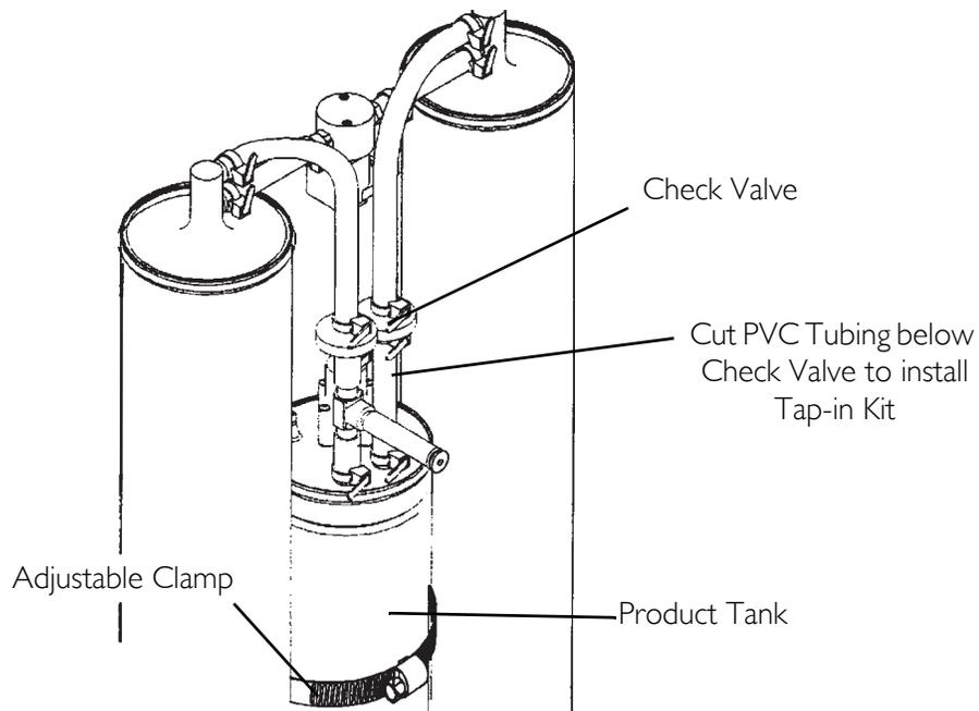
**FIGURE 25.1** Disassembly
