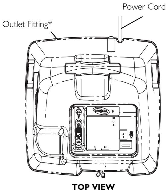
*\*NOTE: This outlet fitting is to be used only for filling oxygen cylinders with the HomeFill II home oxygen compressor. The outlet fitting does not affect concentrator performance. Refer to the HomeFill II owner's manual, part number 1116444, for connection and operating instructions. When not in use, the plug provided with the concentrator should be inserted into the outlet fitting. For more information about the HomeFill II, contact Invacare.*
