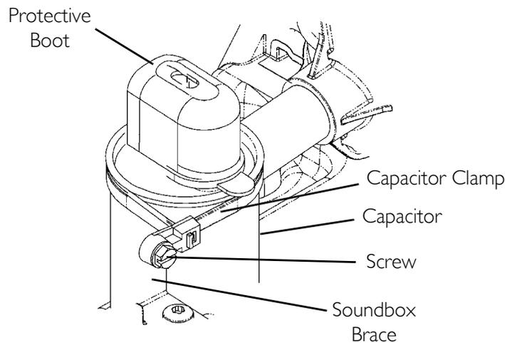
**FIGURE 7.4** Replacing Capacitor
