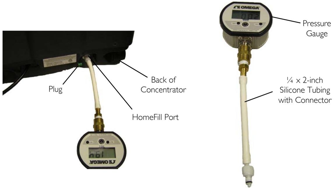
**FIGURE 25.5** Pressure Testing
