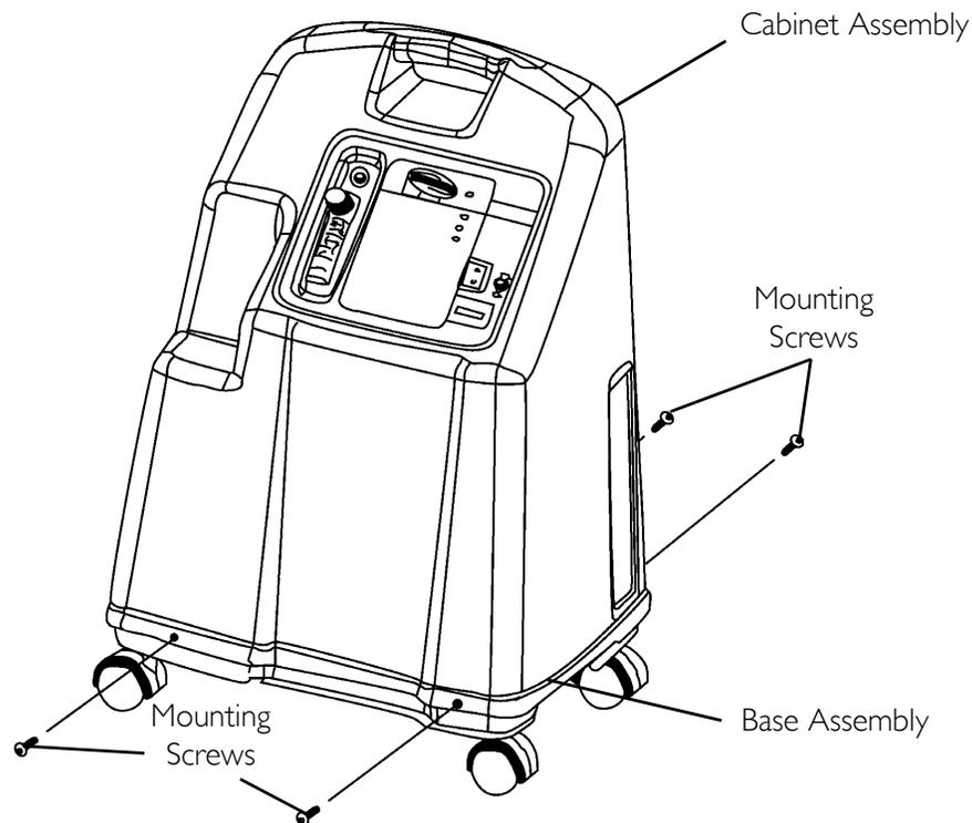
**FIGURE 5.1** Removing Cabinet
