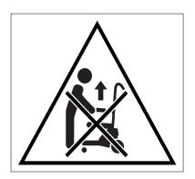
Do not use armrests to lift the device, especially if the person to be conveyed is sitting in the scalacombi. To ensure user-friendliness, the armrests are rotatable and detachable (e.g. for transfer to the seat of the scalacombi) and might be inadvertently pulled off, depending on direction of force.
