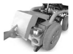
• Remove plastic clips (1) and remove device support upwards to the rear.
