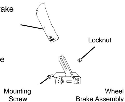
**FIGURE 7.3** Replacing Wheel Brake Handle
