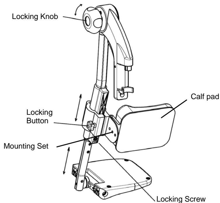
**FIGURE 2.5** Adjusting Elevating Legrest Height and Calf pad Height/Depth
