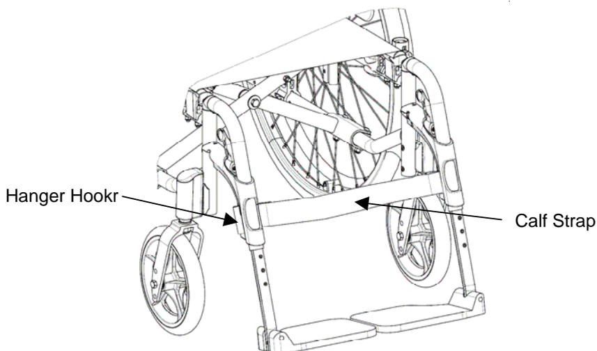
**FIGURE 2.3** Installing Calf Strap
