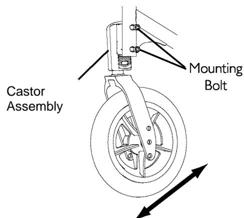
**FIGURE 5.10** Adjusting Castor Angle
