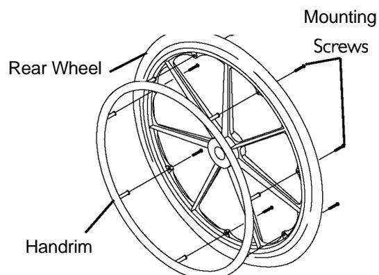
**FIGURE 5.4** Replacing Handrims
