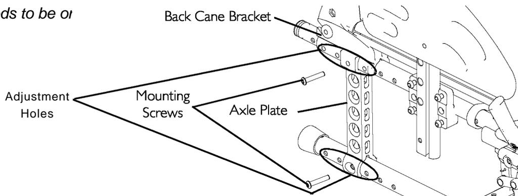
**FIGURE 5.5** Adjusting the Wheelbase Length
