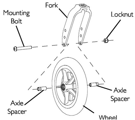
**FIGURE 5.98** Removing/Installing/Repositioning the front wheel
