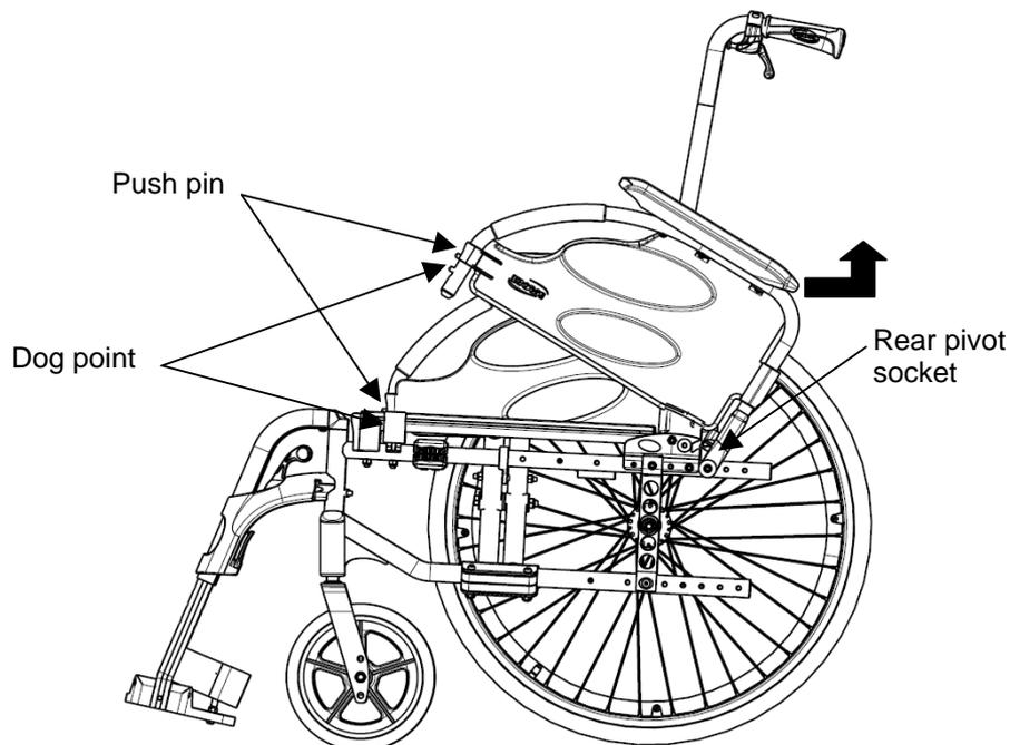
**FIGURE 3.2** Removing/Installing Swing Away Armrest
