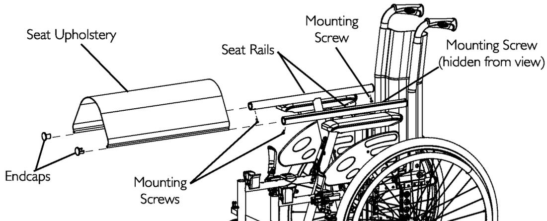
**FIGURE 4.2** Removing/Installing Seat Upholstery
