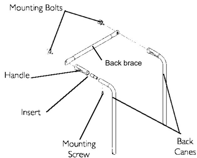
**FIGURE 4.11** Installing/Removing the Back Brace
