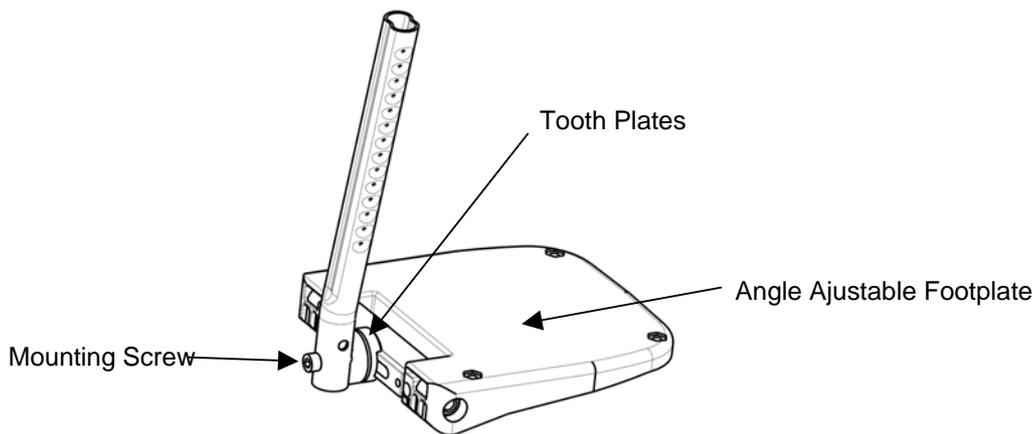
**FIGURE 2.4** Installing Angle Adjustable Footplate
