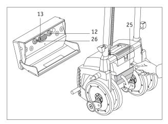
Under no circumstances must you turn the rotary switch to the right of the single-step switch [12]. This was adjusted by the specialist dealer to exactly suit your staircase. Improper adjustment to this switch may result in functional problems with your scalamobil.
