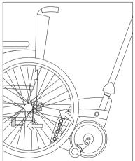
lock the upper holding device [20] with the locking pin [19]. Unlock the locking pin by pushing in its center with your thumb, then drive the locking pin all the way into the holding device.
