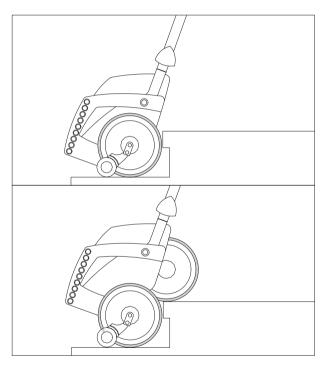
During the climbing process always pull the scalamobil towards you. Also the scalamobil plus wheelchair needs to remain in the same tilted, balanced position all the time. Never release the grips of the scalamobil!
