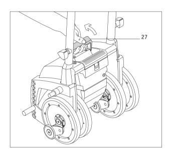
After you have removed the handle as described in the last chapter, you can fold out the carrying handle [27] that is integrated into the housing, in order to be able to transport the scalamobil.
