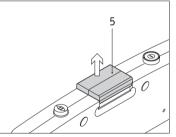
Pull the adjustment button up; safety mechanism is disengaged.
