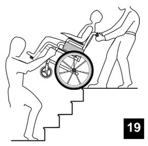
The second helper, holding firmly a fixed part of the front frame, lifts the wheelchair above the stairs and holds it while the first helper places one foot on the following step and repeats the operation.
