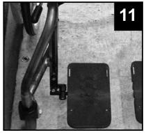
sitting in the wheelchair and should not be used for standing. Each footplate assembly can be adjusted in height. The footplates can be pivoted to an upright position to aid front transfers.
