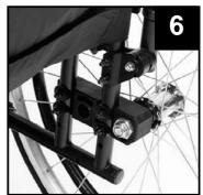
axle though the axle bush, making sure that the axles are secured (no axial movement).
