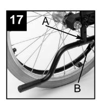
Fit the tipping lever into the side frame rear
