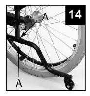
wheelchair even if you do not wish to use them. Just depress the button spring and rotate the entire anti-tipper unit a half turn (180°). DO NOT twist or turn the Anti-Tipper when withdrawing it from the frame.
