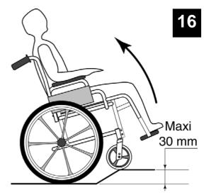
Lower the front of the wheelchair smoothly, holding the handles firmly. Use your weight on the foot step tube to act as a counterweight. Do not lower the wheelchair suddenly down the last few centimetres before returning to the normal position as this may hurt the user.
