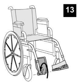
If possible, fold back the footrest supports to the side to clear the passage. (Figure 14)
