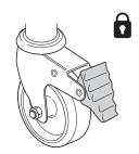
**Locking the brake** - Step on the outer part ® of the brake pedal **Unlocking the brake** - Step on the inner part ® of the brake pedal
