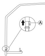
Lift the lifting pole until the control latch  $ext{(A)}$  is released from the lifting pole tube.
