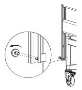
Retighten the screw under the lower side rail bar, in each corner of the bed ends.
