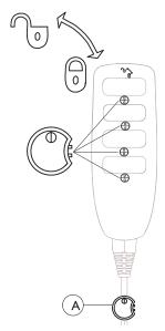
Insert the key (A), in the key hole, below the wanted function and turn it.
