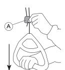
Lock the handle by pressing back the cord in the lock  $\ensuremath{\widehat{\mathbb{A}}}$  and pull the handle downwards.
