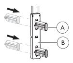
Push the pawl  $\mbox{\@A}$  from the backside, through the glider  $\mbox{\@B}$  and make sure it locks with an audible click.
