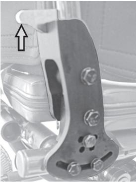
3. Pull up on the trigger mechanism for the backposts and push the backposts to the flat position over the seat rails.
