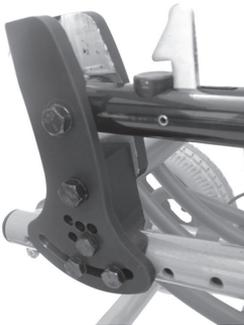
3. Unfolding the back assembly is accomplished by grasping the push handles or straight back posts and pulling them to an upright position where they will lock into place.
