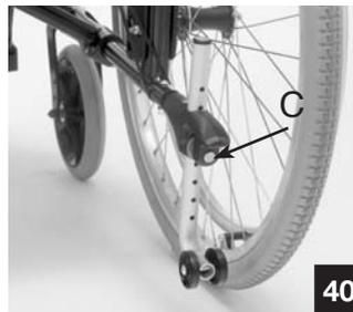
Push down the button (C in photo 39 & A in figure 41) and adjust the wheels holding tube for the desired distance based upon the preset holes.
