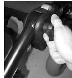
Turn the knob clockwise to tighten it.
