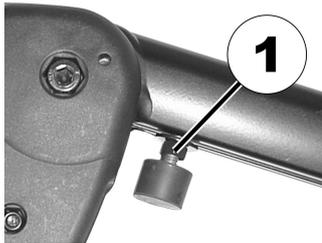
Use the open-ended spanner to loosen the counter nut (1).
