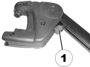
The end position of the legrest is determined by means of a rubber stop (1).
