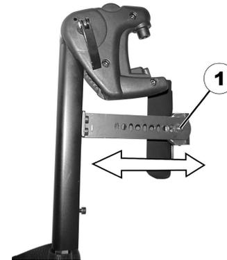
1. Use the open-ended spanner to loosen the nut (1) and remove.
