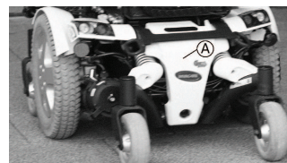
Ⓐ Power module behind rear shroud
