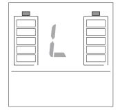
When activating the button lock, the following is shown in the display: the current charge status of the two battery packs, an  $_{\mu}L^{\mu}$  in alternating fashion, the power stage currently set (1 or 2) and in case an error occurs, the corresponding error code.
