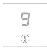
If the remote control does not detect the two wheels (for example, due to a poor remote communication), the information message shown here appears on the display.
