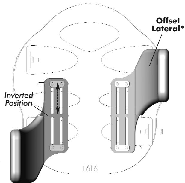
**\*note:** offset laterals may also be mounted in the inverted position (as shown) to provide extended support
