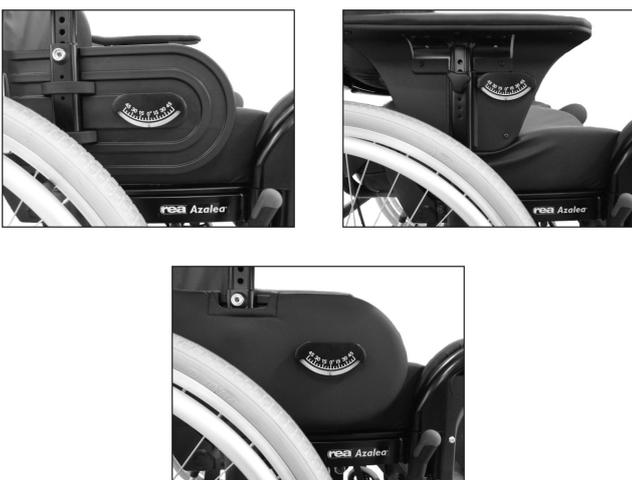
The tilt scale for the seat angle, is placed on the armrest according to the pictures above.
