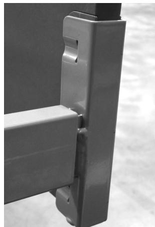
For the Vibeke bed end, insert the separate brackets for the bed ends into the side tube of the mattress platform and tighten the screws firmly with a 5 mm Allen Key. Lower the bed end board in the U-bracket fitting and press down firmly to ensure that bed end is fully seated at bottom of U-bracket fitting.
