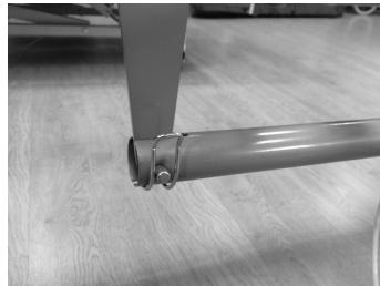
Join the backrest crank/tube with the backrest bracket, using a pipe pin in the hole of the bracket.
