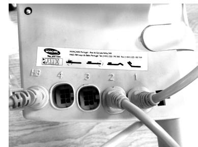
Connect the section motor wires to the control box.
