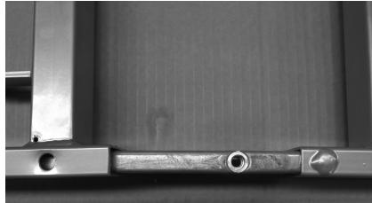
Place the two inserts in the head end of the mattress support and push the ends together.
