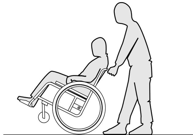
To show the user the tipping point, the wheelchair can be tilted backwards by an assistant using the push bar.
