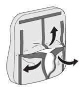
4. The Laguna pad has Velcro strips on the back of its cover and is inserted into the plastic shell casing in the place where the standard pad is otherwise fitted. The pad's cover can be removed and washed according to the washing instructions. Remove the cover by unzipping it and pulling it off the pad.
