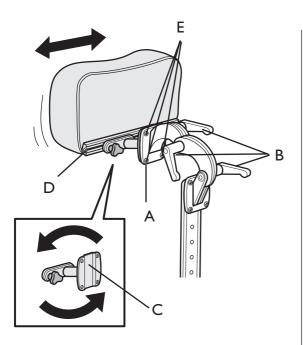
To adjust the neckrest/headrest sideways loosen the knob/screw (A). Adjust to a new position and tighten the knob/screw (A). Adjust the angle and height by loosen the handles (B). Change to a new position and tighten the handles (B).
