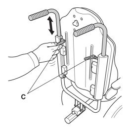
1. To replace the push bar with a push handle bar, you must first remove the handles for the backrest tilt and the seat tilt adjustments. The tilt handles must be moved from the push bar to the push handle bar.
