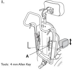
I. You adjust the trunk support attachment by loosening screw (A) using a 4 mm Allen key.Adjust to the position that you require and retighten the screw.
