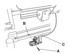
Start by removing the standard rear wheel brake. Attach the one-arm brake to the suitable side of the chair by tightening screw (A) in the existing square nut (B).
