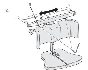
2. Adjust the legrest to a central position by loosening both Allen screws (B) as shown in the picture. When you have found the desired position, retighten the screws.
