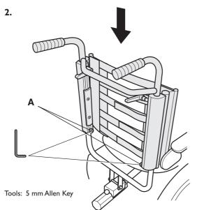
3. B Tools: 5 mm Allen Key  Start by removing the push bar or the push handle bar. Then remove the existing backrest by loosening both of the lower screws (A).
