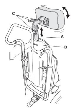
You adjust the height of the central support (A), by loosening handwheel (B), adjusting to the desired height and retightening. The angle and height of the neck rest are adjusted by loosening the levers (C). Change to the desired position and retighten the handwheels.
