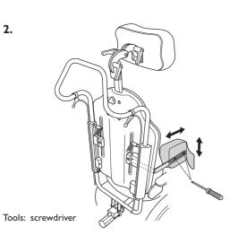
2. You can open the trunk support pad using the zip. You can then adjust the trunk support by loosening the two screws using a Phillips screwdriver and moving the trunk support forwards or backwards. Retighten the screws and close the zip.
