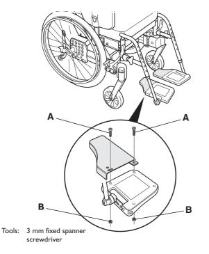
Fit the extension to the foot plate using the screws (A) and nuts (B).
