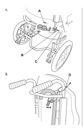
Fit the crutch holder attachment around the backrest tube using the screw (A), washer (B) and nut (C).
