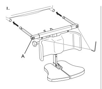
If you want to fit a central legrest to the wheelchair, you must first remove the existing seat extension. Use an Allen key to loosen both screws (A). Then fit the central legrest, set the required seat depth and tighten the screws (A).
