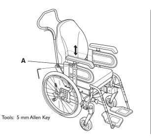
Adjust the height of the armrest using screw (A).
