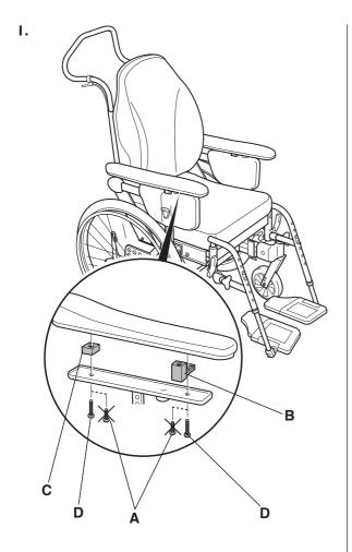
Loosen the screws (A) on the underside of the armrest. Remove the armrest pad. Fit the table tray's attachment casing (B) and spacer block (C) between the armrest pad and its attachment plate. Attach the armrest pad with the new screws (D).
