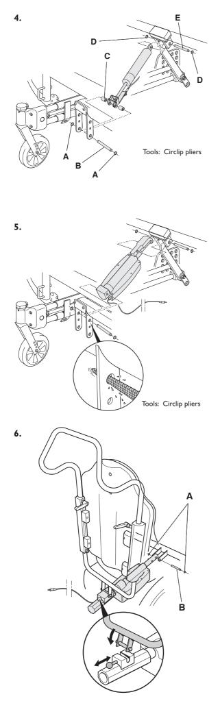
4. Remove the frontal seat tilt piston by loosening the circlips (A) and removing the dowel (B), the spacers (C) and then loosening the circlips (D), removing the dowel (E) and loosening the piston from its attachment at the rear of the chair.
