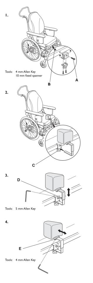
I. Fit the pommel attachment to the front of the chair using the screw (A) and nut (B).
