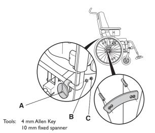
Fit the red reflector on the back of the backrest tube using the screw (A), washer (B) and nut (C). Attach the orange reflector to the spokes of the rear wheels, by placing both clips (D) at a suitable distance from each other, each of them around a spoke, and then pushing the reflector onto it.
