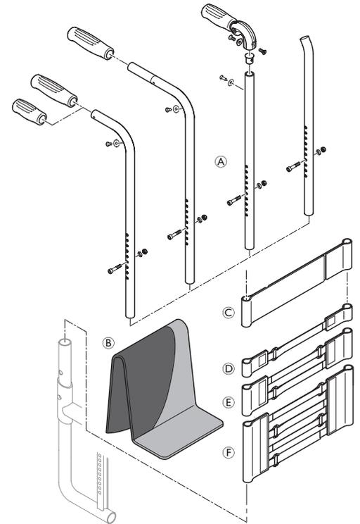
\*Stabilization bar not possible for foldable push handles
