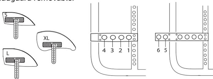
*Mudguard (removable) with respect to the position of the rear wheels with standard adapter plate (Pos. 1 to 4) or rear wheel extension (Pos. 5 and 6)*
