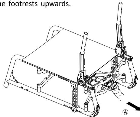
3. Push on the black plastic handle on the front or pull the black plastic handle **A** on the rear of the wheelchair.
