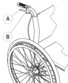
1. To brake, pull the brake lever **A** on the push handle.
