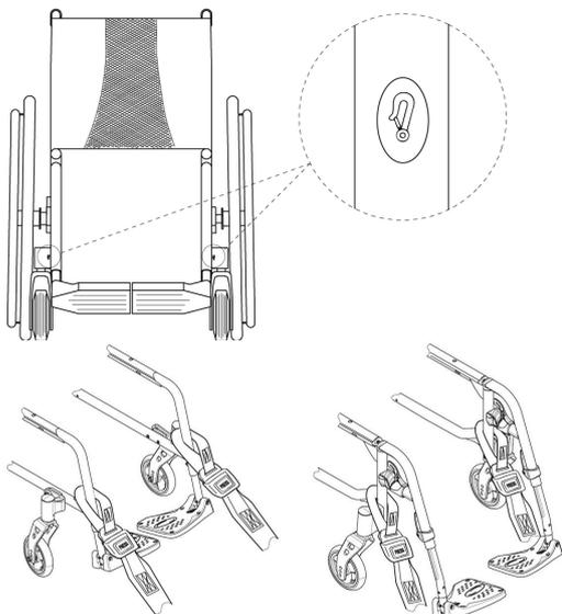
1. Attach the front straps above the castor supporters as shown in the two figures above (see location of the attachment labels).
