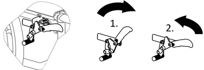
1. To engage the brake, push the brake lever forwards with the palm as far as possible.
