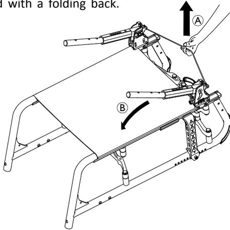
6. Pull the pull-cord **A** upwards at the back of the wheelchair. The backrest **B** folds forwards.
