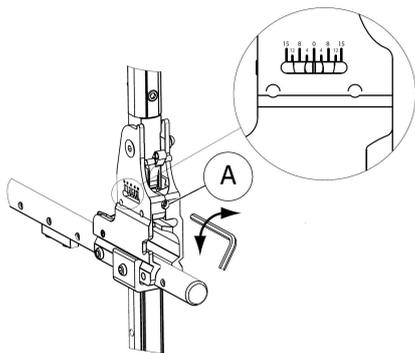
1. Adjust the backrest angle thanks to the adjustable screw (A).
