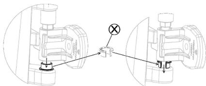
1. Extract the grey spacer open ring **X** out of its location.
