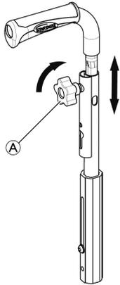
1. To set the height of the push handles, loosen the knob **A**, push the handle to the desired position and tighten the knob again.
