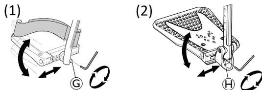
1. Loosen the fixing screw ⑥ or ⑧ with 5 mm Allen key.
