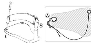
The plastic buckle must be fitted facing outwards and as close as possible to the tube of the footplate ①.
