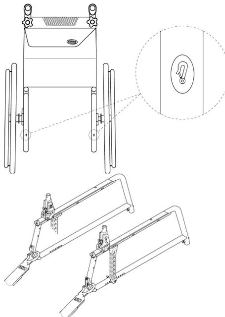
1. Attach the snap hooks to the rear frame right above the adapter plate as shown in the two figures above (see location of the attachment labels).
