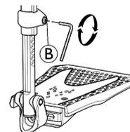
1. Loosen the fixing screw **B** with 5 mm Allen key.
