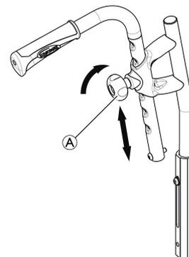
1. To set the height of the push handles, loosen the knob (A), push the handle to the desired position and tighten the knob again.
