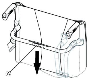
1. Unlock the folding backbrace by pushing the joint (A) slightly downwards.
