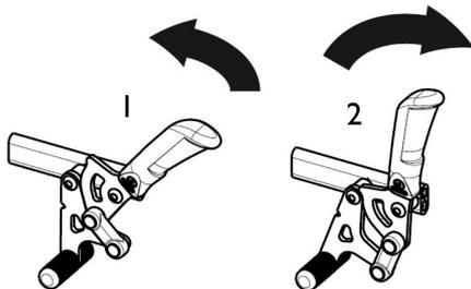
1. To engage the brake, pull the brake lever backwards with the low fingers as far as possible.
