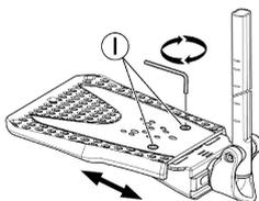
1. Loosen the two fixing screws ① with 5 mm Allen key.
