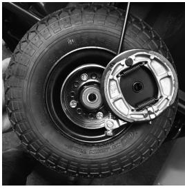
Pull brake out of brake drum.
