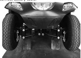
Place a supporting wooden block under the front part of the frame so that the front wheel is no longer touching the floor.
