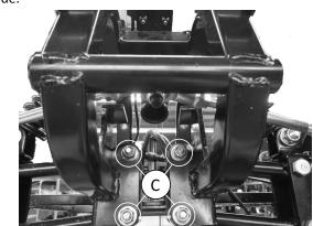
Loosen four screws © that fix cross members to frame.
