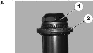
Loosen wheel suspension screw (1).
