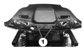
Remove screws (1) on brake light.
