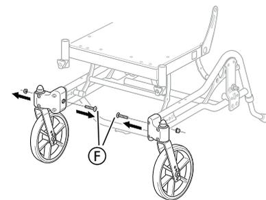
9. Loosen the screws to the castor attachment (F).
