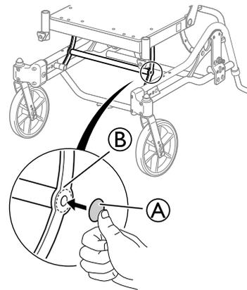
Add the first sealing stickers **A** over the holes of the cross tube **B** on both sides.
