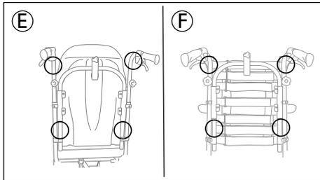
Place the tilt scale for the backrest angle on the push bar/push handle or on the backrest tubes according to picture **E** or **F** above.
