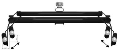
The backrest tubes have a width adjustment of 25 mm. The upper and lower parts of the tubes can be adjusted individually to accommodate for different needs. The outward movement will embrace the user and offer lateral support.
