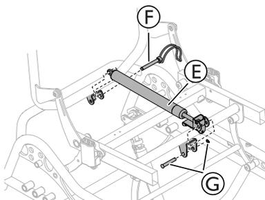
1. Assemble the gas piston **E** to the front and the rear attachment.
