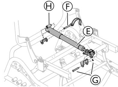
3. Assemble the gas piston **E** to the front and the rear attachment.
