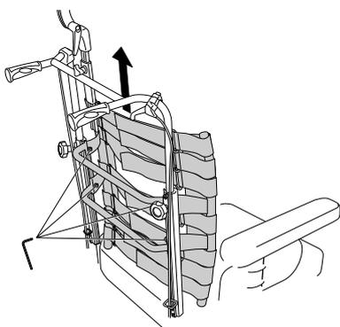
Loosen screws and remove the backrest by lifting upwards.
