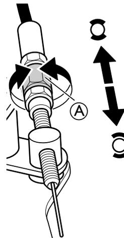
Adjust the brake effect with the adjustment nut **A** on the wire.
