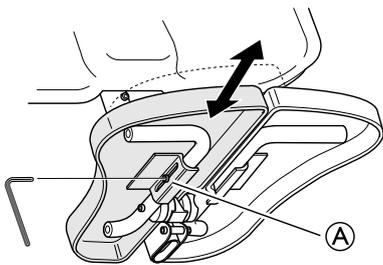
1. Loosen the frontal screw (A) on the side of the tube.
