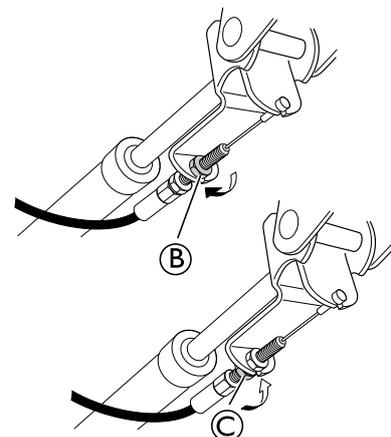
Fixate the wire in the holder with the fixation nut (B). When the desired tilt resistance is achieved, fixate the position with the fixation nut (C).
