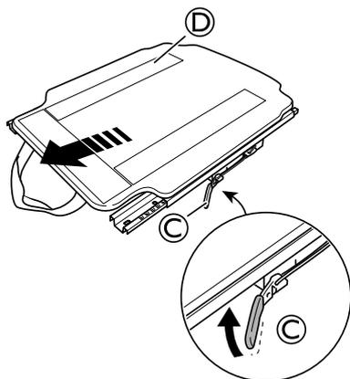
Press the release handle **C** and push the sliding seat **D** forwards.
