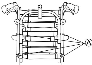
1. Loosen the four screws (A) as shown above.
