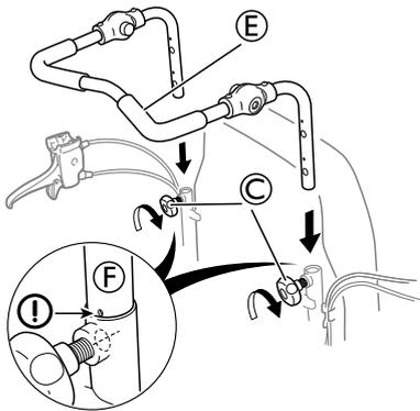
Mount the push bar (E) in the backrest tubes and tighten the handwheels (C).
