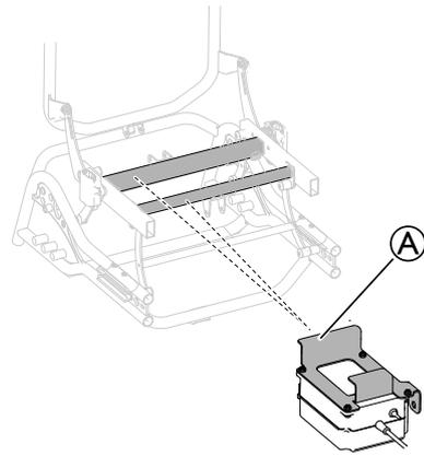
1. Mount the attachment with the battery ① on the frame.
