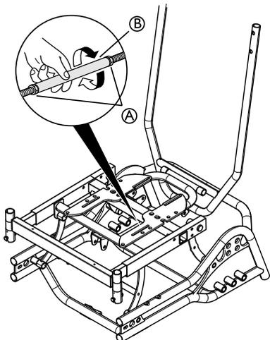
1. To adjust the angle of the backrest, first loosen nuts (A) on the rigging screw.
