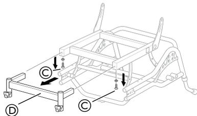
3. Loosen and remove the screws (C).
