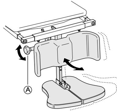
1. Loosen the adjustment knob (A).
