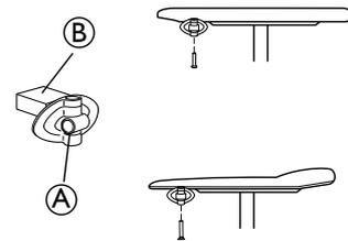
Mount the table attachment **A** with the attachment part facing outwards. The plain surface **B** of the attachment should be placed upwards when using the table on the thin armrests.
