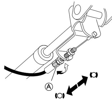
Adjust the tilt resistance with the adjustment nut (A) on the wire.
