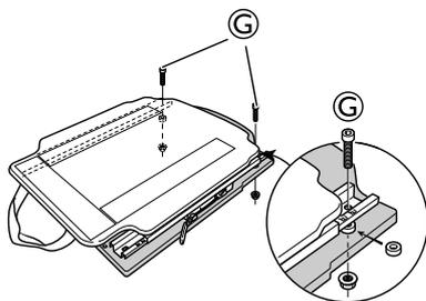
Attach and tighten the rear screws and nuts **G**.
