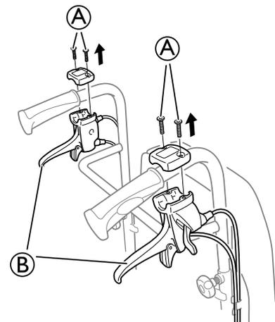
Loosen and remove the screws **A** and the brake handles **B**.
