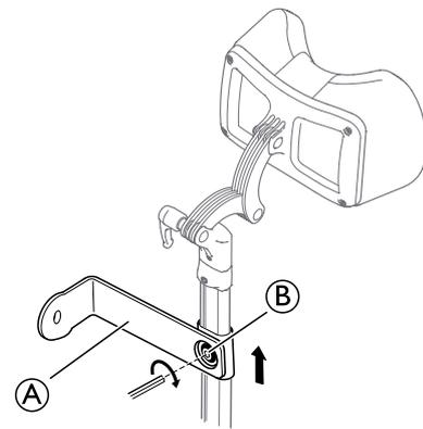
Mount the holder for the drip stand (A) on the neckrest holder and tighten the screw (B).
