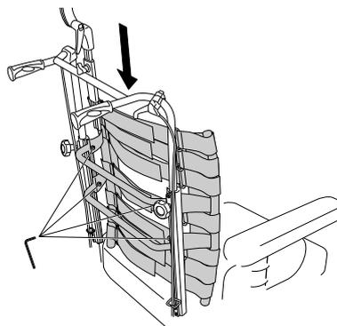
Put the backrest back by fitting it to the receivers on the tubes. Tighten the screws.
