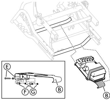
1. Mount the attachment ② with the attached control box on the chassis.
