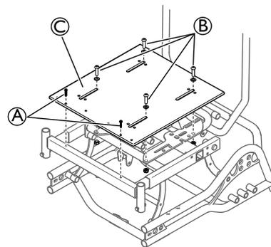
**i** The seat plate can either be used as a base for a seat cushion or for attaching seat shells and other seating modules.
