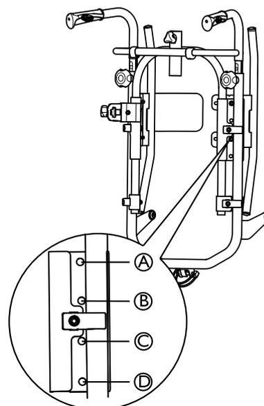
(A) to (D) Screws for alternative height adjustment
