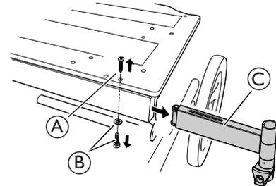
Remove the upper screw (A) and the lower screw and washer (B). Remove the ordinary legrest attachment (C).
