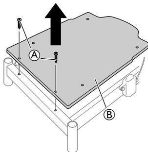
1. Loosen and remove the screws ① and the seat plate ②.
