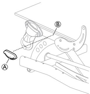
Place the tilt scale for the seat **A** on the seat frame **B**.
