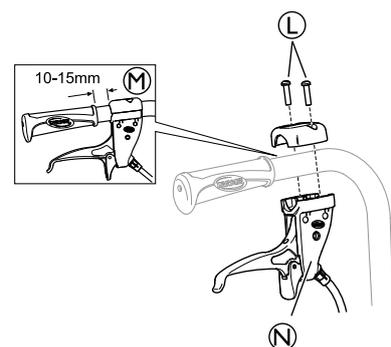
Mount the lever for the assistant maneuvered drum brake **A** on the push handle and attach the screws **B**.
