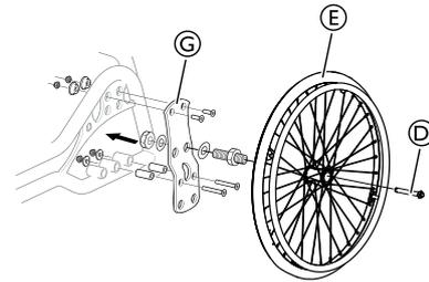
1. Attach the new rearwheel plate **G** and the screws, nuts and sleeves.
