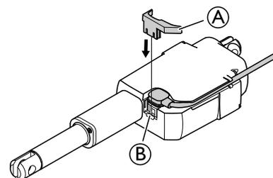
1. Place the cable in the holder © on the seat tilt actuator.
