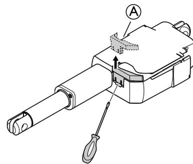
1. Loosen the cable lock (A).
