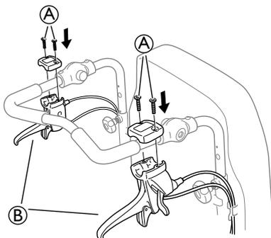
Re-mount the brake handles (B) and tighten the screws (A).
