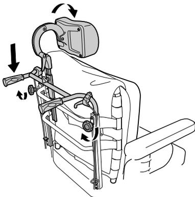
Lower the push handles and tighten the hand wheels.
