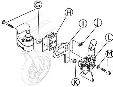
2. Mount the new transport attachment and the fixation ① and ②.
