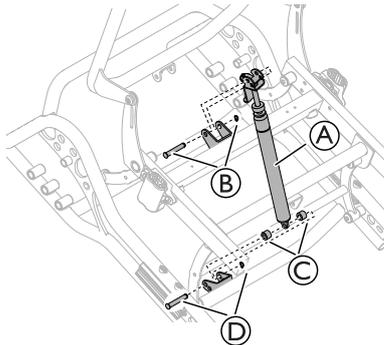
1. Assemble the gas piston **A** to the front and the rear attachment.
