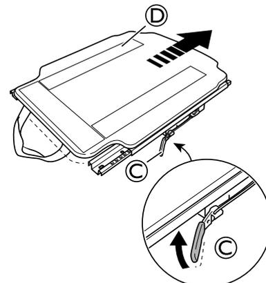
Press the release handle **C** and push the sliding seat **D** backwards.
