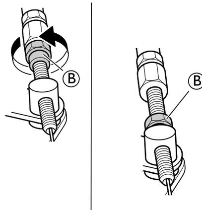
When the desired brake effect is achieved, fixate the brake wire with the fixation nut **B**.
