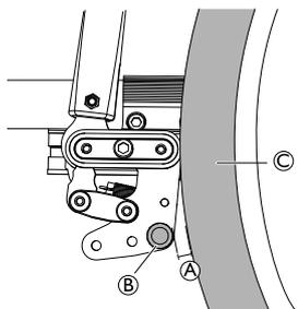
**i** The distance **A** between the pin **B** and the tire **C** should be max. 15 mm.
