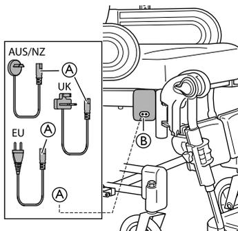
1. Connect the charger cable supplied with the chair into a wall socket.
