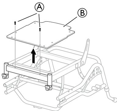
1. Loosen and remove the screws (A).
