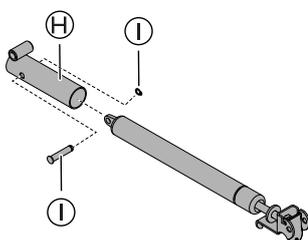
1. Assemble the gas piston attachment **H** on the gas piston.
