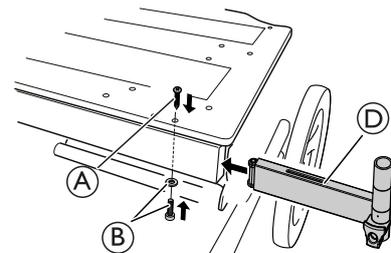
Mount the high legrest attachment (D) in the seat frame. Re-insert the upper screw (A) and the lower screw and washer (B). Re-tighten the screws.
