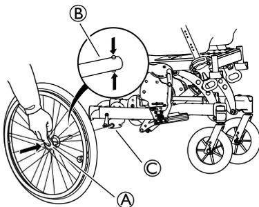
1. Press and hold in the quick-release button (A).
