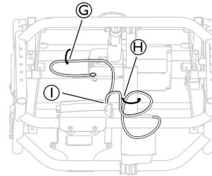
1. Attach the cable for the seat tilt (G) to the frame with a cable tie.
