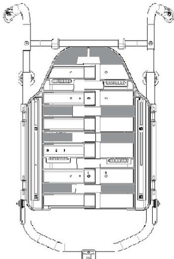
1. Remove the width adjustment plates.
