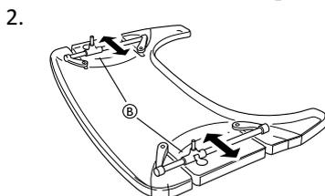
Adjust the attachment bars (B) in order to fit the table to the desired width. Re-tighten the screws.
