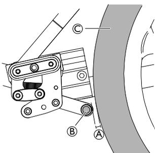
**i** The distance **A** between the pin **B** and the tire **C** should be max. 6 mm.
