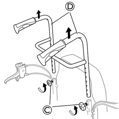
Loosen the handwheels **C** and remove the push handles **D**.
