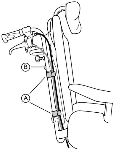
1. Thread the wires on the outside of the backrest tubes **B**.
