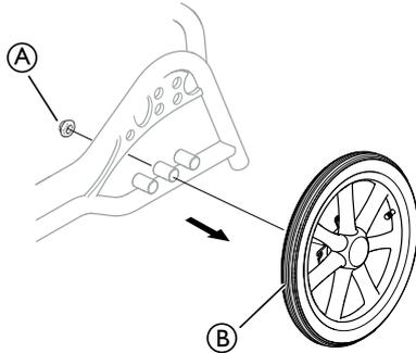
1. Loosen and remove the nut **A**.
