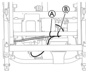
1. Attach the cable for the battery charger (A) and for the battery (B) to the frame with two separate cable ties.
