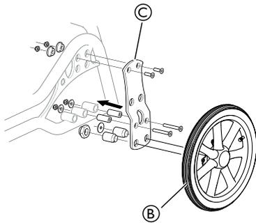
1. Attach the new rearwheel plate **C** and the screws, nuts and sleeves.
