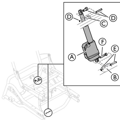
1. Place the upper part of the piston for the tilt (A) in the attachment © on the frame.
