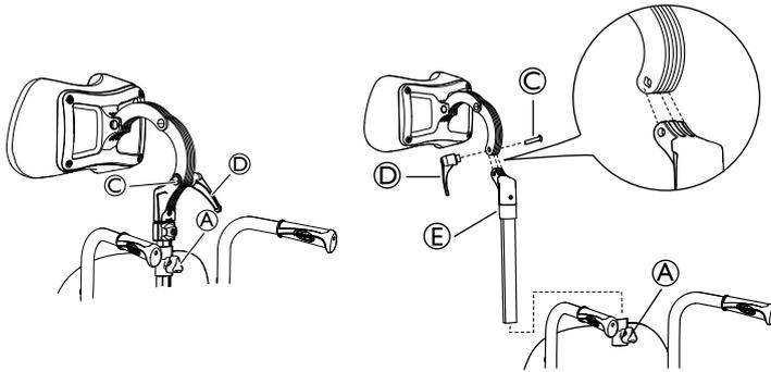
**i** You can also adjust the angle and depth by turning the attachment for the headrest / neckrest.
