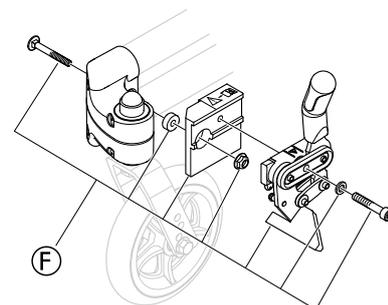
1. Remove and scrap the castor locking and the screws and nuts ⑥.
