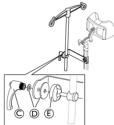
Mount the lever (C), the washers (D) and the holder with the drip stand (E) in the attachment and tighten the lever.
