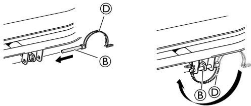
3. Close the safety shackle (B) with the lock shackle (D) to secure the Rigging screw (A).
