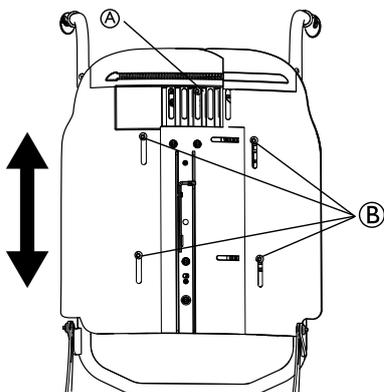
(A) Upper screws for additional height adjustment
