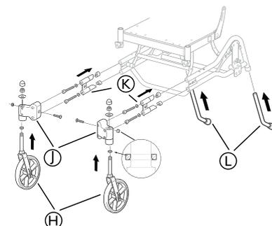
13. Mount the chassis extenders (K) on the chassis tubes.
