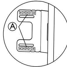
The backrest tubes can be angled individually, the indication labels (A) on the backrest tubes are a help in order to get the same angle on both sides.
