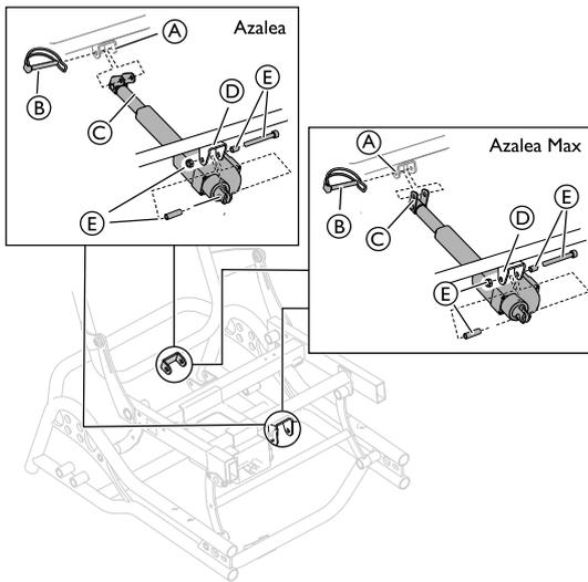
1. Place the attachment to the piston for the backrest recline © in the attachment (A) on the frame.
