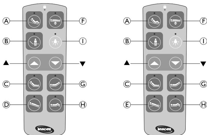
The hand control is equipped with buttons for electrical functions (A to H), up and down buttons (▲ and ▼) to control the selected function and optionally with a button for an under bed light (I).
