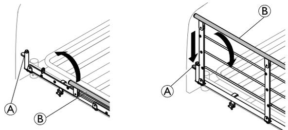
1. **Up:** Lift and pull the top bar **B** of the side rail towards the end with the locking mechanism (release button) **A**. Ensure, it is locked in place.
