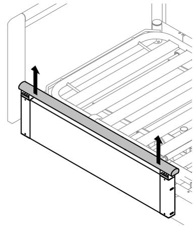
Pull the top bar upwards with both hands near the left and right end.
