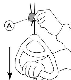
1. Hold the cord out while sliding the plastic cord lock (A) upwards or downwards until the handle reaches the preferred height.
