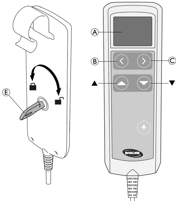
1. Turn the safety key **E** to the unlocked position.
