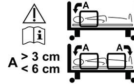
Indicates the allowed mounting positions and spaces between the side rails and the bed ends, when only one side rail is mounted on the side of the bed or when two side rails are mounted on the same side of the bed.
