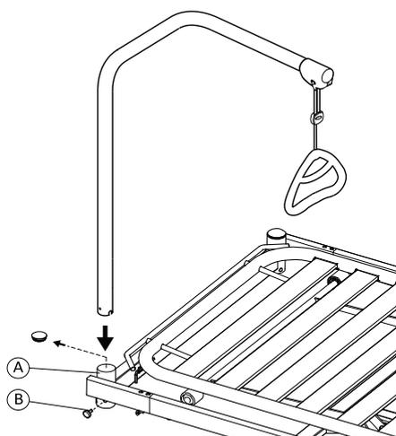
1. Remove the plastic plug from the lifting pole tube (A) at the head end of the bed.
