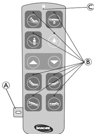
1. Insert the magnetic key (A) in the slot on the side of the hand control.
