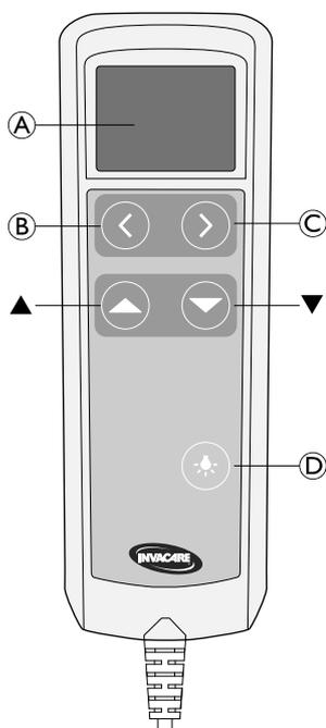
The hand control is equipped with an LCD display (A), navigation buttons (B and C) to select the electrical functions and up and down buttons (▲ and ▼) to control the selected function.
