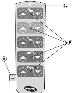
1. Insert the magnetic key **A** in the slot on the side of the hand control.
