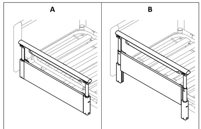
To raise the side rail to the middle position (A), stop pulling upwards after a first audible click.
