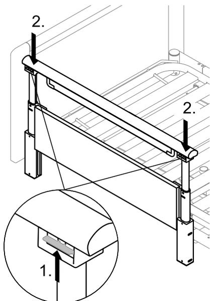
1. Push up and hold the two release buttons.
