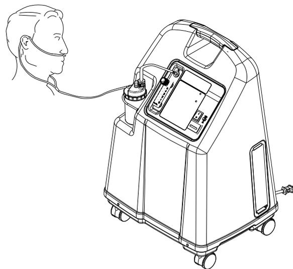
Fig. 3-2 Concentrator with Humidifier
