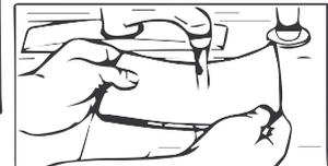
1. Remove the filter (A) and clean as needed.
