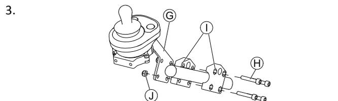
Attach bracket **G** to gripper clamp **I** with screws **H** and nuts **J**.
