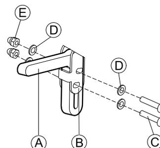
Mount joystick holder ① to remote adapter ② with screws ③, washers ④ and nuts ⑤.
