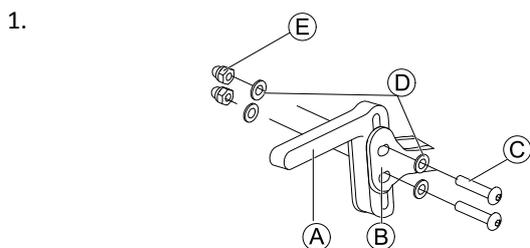
Mount joystick holder (A) to remote adapter (B) with screws (C), washers (D) and nuts (E).
