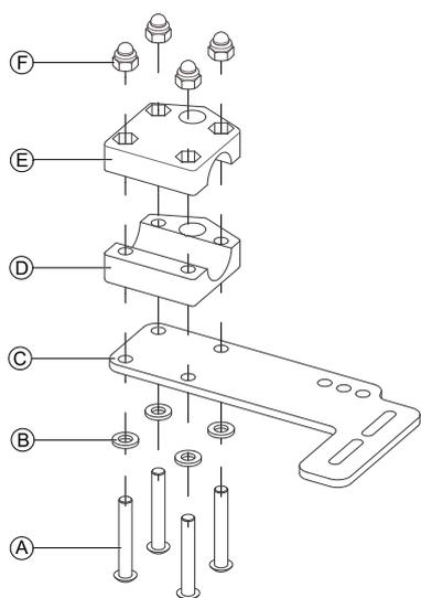
1. Pull screws ① through washers ②, mounting plate ③ and bottom side of bracket ④.
