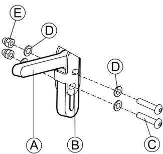
Mount joystick holder **A** to DLX-CR400 adapter **B** with screws **C**, washers **D** and nuts **E**.
