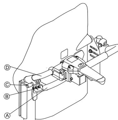
1. Fix the retaining clamp **B** on the wheelchair push handle **A**.
