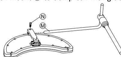
Pull hitch mount over nucleus (M) and tighten with screw (N).
