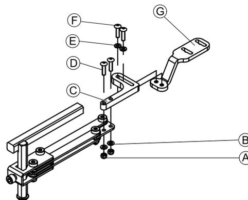
1. Pull screws (D) through bracket (C), remote holder and washers (B).
