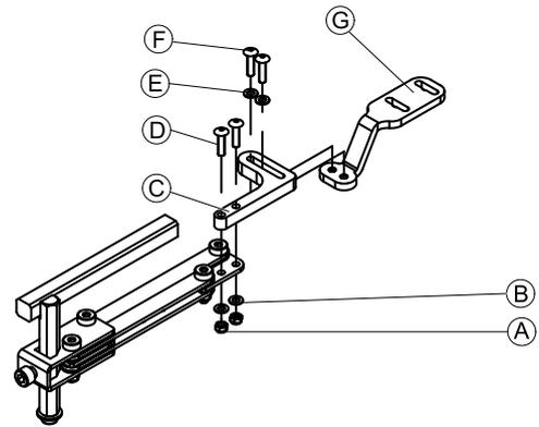
1. Pull screws **D** through bracket **C**, remote holder and washers **B**.
