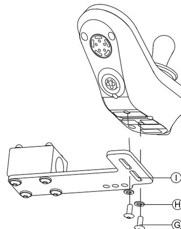
Fix remote to bracket ① with screws ③ and washers ④ .
