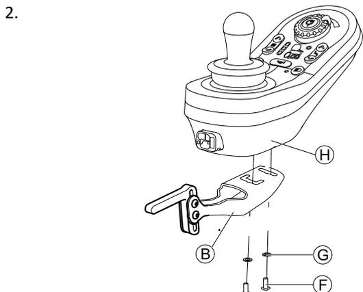
Mount remote (H) to remote adapter (B) with screws (F) and washers (G).
