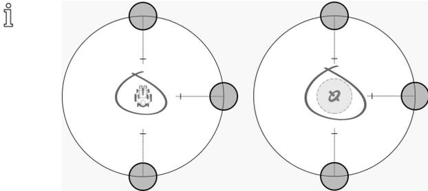
If a gyro module is enabled, the graphic in the center of the graph changes from a person in a wheelchair to a gyroscope to indicate that the parameter being changed are gyro-specific.
