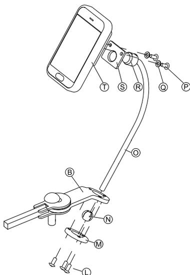
Insert bracket **O** into joint arm **B**, clamp ball **N** and clamp ring **M**.
