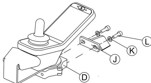
Attach clamp **D** to bracket **J** with screws **L** and washers **K**.
