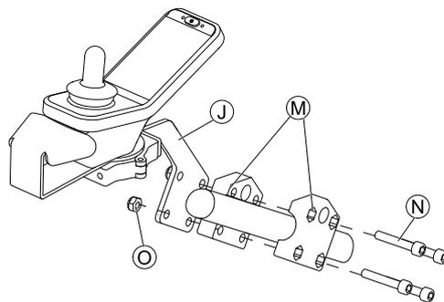
Attach bracket **J** to gripper clamp **M** with screws **N** and nuts **O**.
