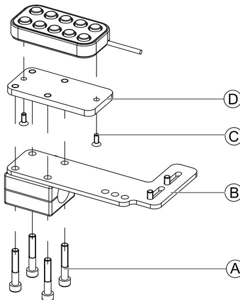
1. Tighten 10 way switch to mounting plate D with screws C.
