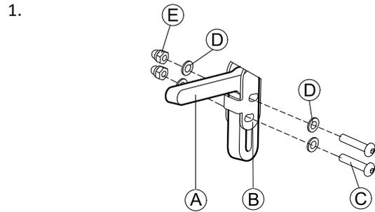
1. Mount joystick holder (A) to remote adapter (B) with screws (C), washers (D) and nuts (E).
