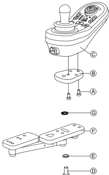
1. Mount LiNX remote adapter ② with screws ① to remote ③.
