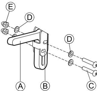
Mount joystick holder **A** to remote adapter **B** with screws **C**, washers **D** and nuts **E**.
