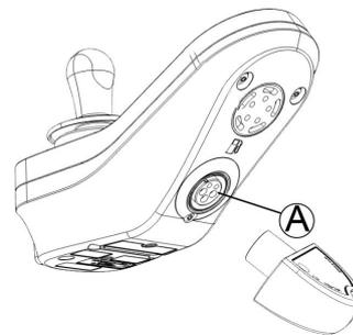
The LiNX Access Key plugs directly into the remote module’s XLR port (A). REM2xx displayed in picture, works for REM400 and REM500 the same way.
