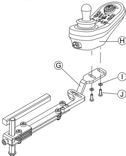
Tighten remote ⑧ with screws ⑩ and washers ⑨ to bracket ④.
