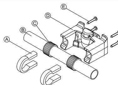
1. Position the tightening clamps **A** on the wheelchair push handle **B**.
