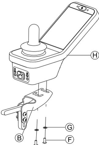
Mount remote **H** to remote adapter **B** with screws **F** and washers **G**.
