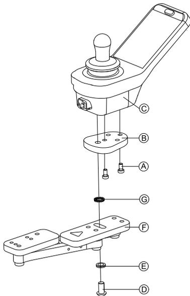
1. Mount LiNX remote adapter **B** with screws **A** to remote **C**.
