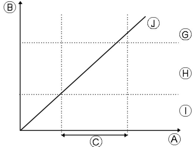
When setting **Sip and Puff Ramp Time**, consideration should be given to users, who cannot produce a hard sip or puff within the ramp time. If ramp time is set too low, a user may not be able to reach the hard zone **G** in time and a soft sip or puff is registered instead of the intended hard sip or puff. For users who need more time to reach hard zone, the ramp time **C** needs to be extended, so the pressure input **I** is registered as a hard sip or puff.
