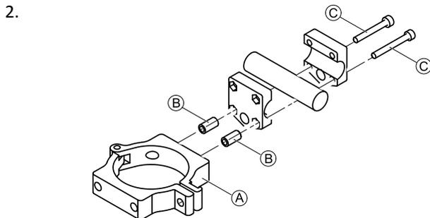
Attach clamp **A** and spacers **B** to gripper clamp with screws **C**.
