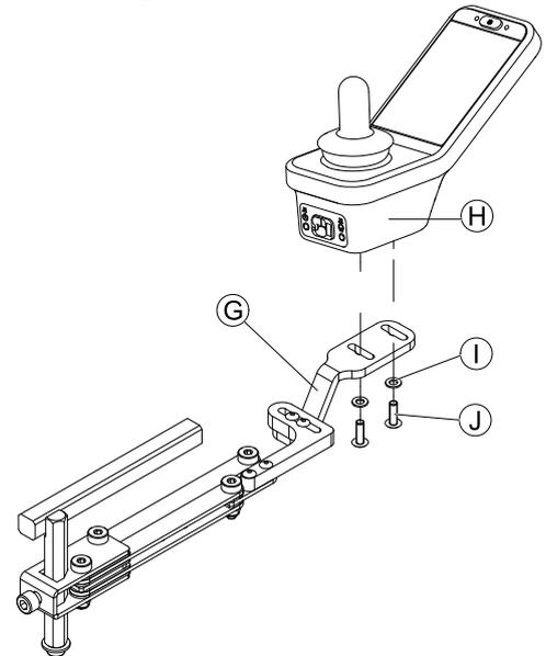
Tighten remote with screws **A** to bracket **G**.
