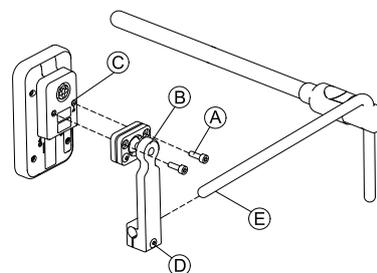
1. Mount remote **C** to bracket **B** with screws **A**.
