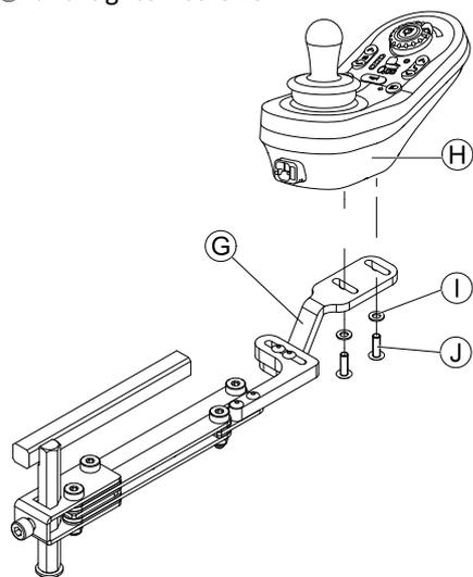
Tighten remote ⑧ with screws ⑩ and washers ⑪ to bracket ③.
