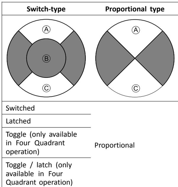
Choose one of the switch-type modes to operate the motion at a fixed speed. The motion is activated when the joystick is deflected past the **Joystick Switch Threshold** **B** into either the forward **A** or backward **C** quadrants. See 8.9 *Joystick Switch Threshold*, page 74 how to modify the **Joystick Switch Threshold**.
