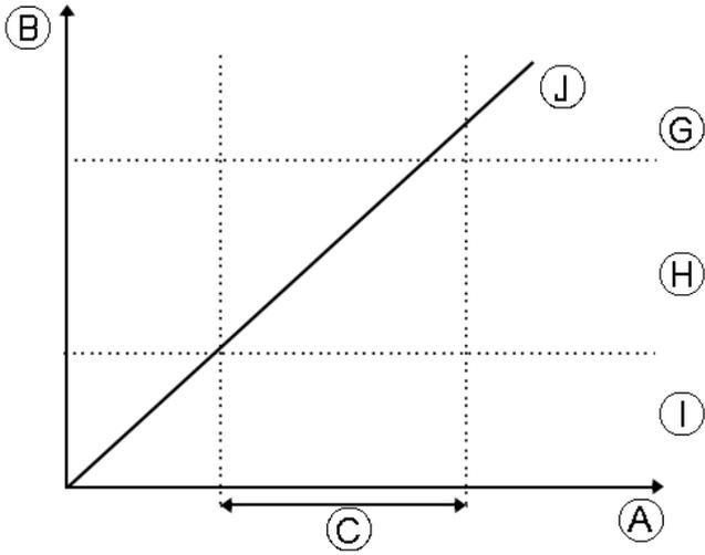
When setting **Sip and Puff Ramp Time**, consideration should be given to users, who cannot produce a hard sip or puff within the ramp time. If ramp time is set too low, a user may not be able to reach the hard zone **G** in time and a soft sip or puff is registered instead of the intended hard sip or puff. For users who need more time to reach hard zone, the ramp time **C** needs to be extended, so the pressure input **I** is registered as a hard sip or puff.
