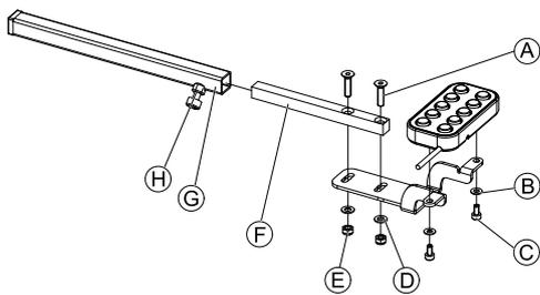
1. Tighten 10 way switch to bracket with screws C and washers B.
