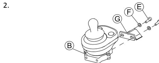
Attach clamp **B** to bracket **G** with screws **E** and washers **F**.
