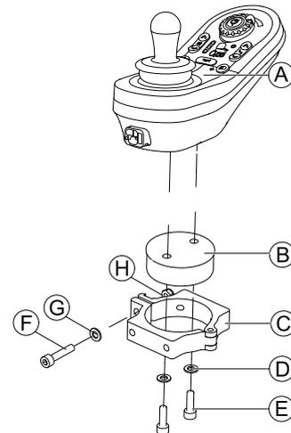
Mount remote ① with and support drum ② to clamp ③ with screws ⑤ and washers ④.
