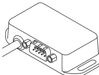
The 4-way button switch or the 4-way toggle switch must be plugged into the DB9 socket.
