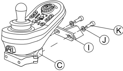
Attach clamp **C** to bracket **I** with screws **K** and washers **J**.
