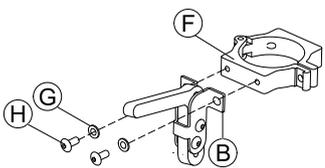
Attach clamp **F** to DLX-CR400 adapter **B** with washers **G** and screws **H**.
