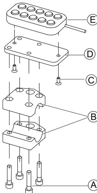
The 10 way switch is fitted to the rear of the wheelchair using a bracket B on the push handle or push bar.
