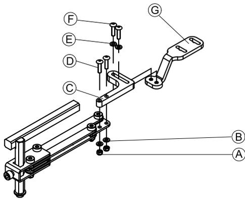
1. Pull screws ④ through bracket ③, remote holder and washers ②.
