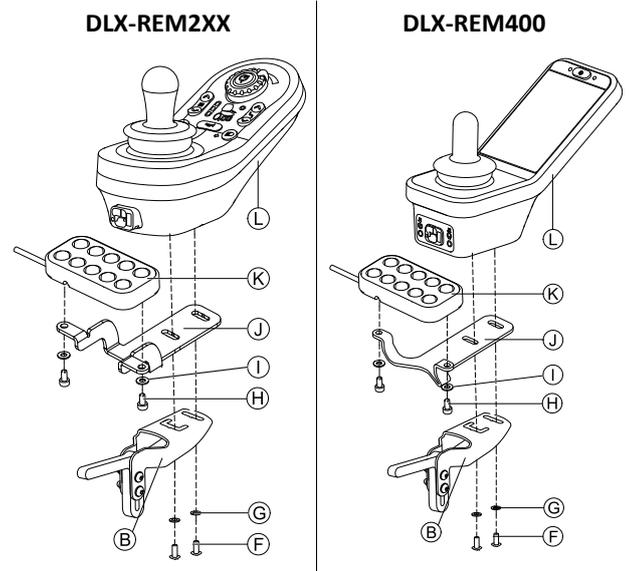
Mount remote (L) to remote adapter (B) and support sheet (J) with screws (F) and washers (G).
