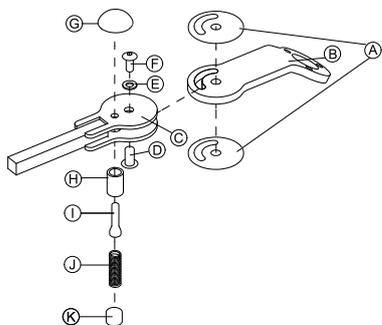
1. Connect slip sticker **A** with joint arm **B** and insert into support **C**.
