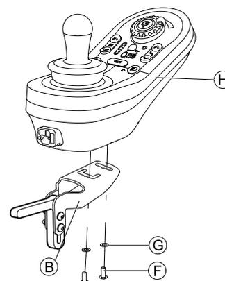
Mount remote ⑧ to remote adapter ② with screws ⑥ and washers ⑦.
