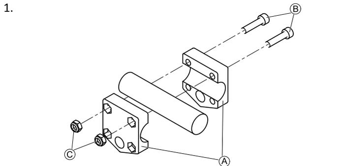
Attach gripper clamp **A** to tube with screws **B** and nuts **C**.
